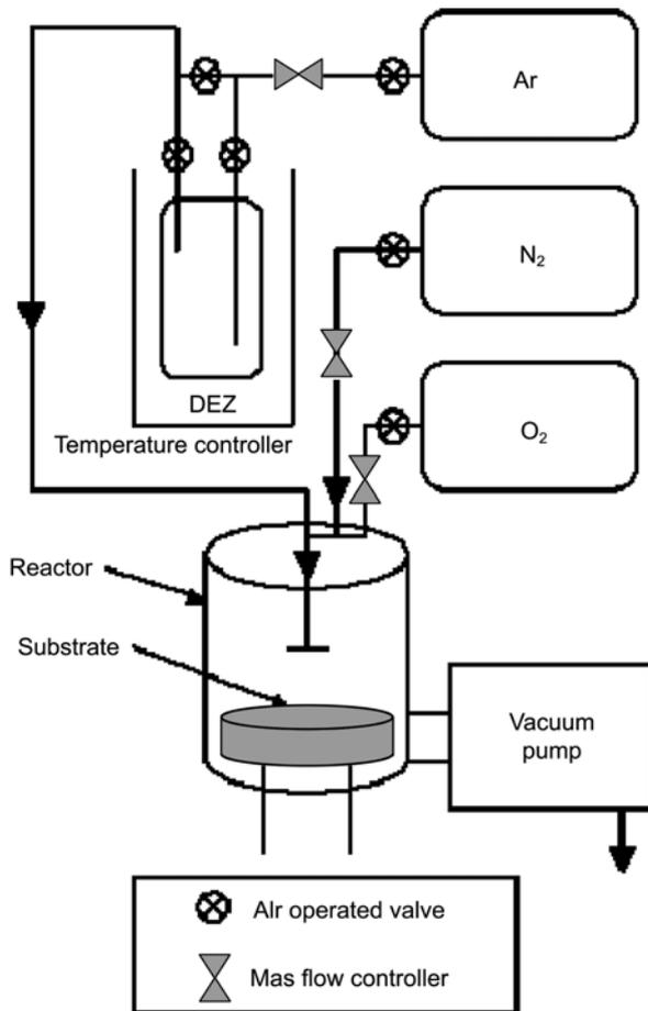
Fig. 1. Schematic diagram of MOCVD system.
