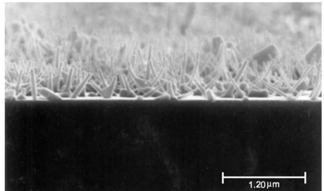
**Fig. 6.** SEM images of ZnO films deposited at 500 °C.
