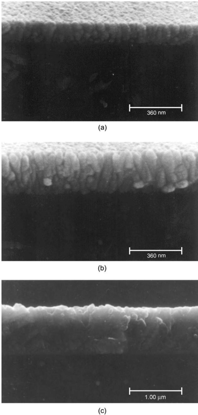
**Fig. 4.** SEM images of cross-section of ZnO films deposited at an Ar/O<sub>2</sub> ratio of 1: (a) 250 °C; (b) 300 °C; and (c) 400 °C.
