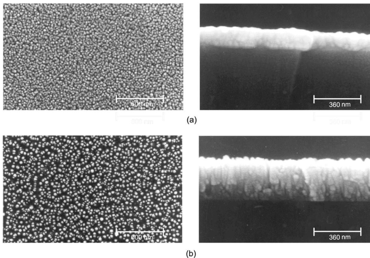
**Fig. 3.** SEM images of top view (left) and cross-sectional view (right) of ZnO films deposited at an Ar/O<sub>2</sub> ratio of 2: (a) 250 °C; (b) 300 °C; and (c) 400 °C.
