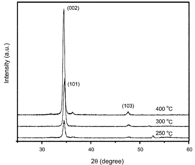
Fig. 2. XRD patterns of ZnO thin films with varying growth temperatures.
