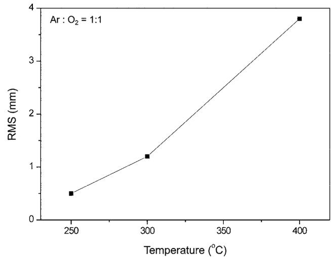
**Fig. 5.** Root mean square data measured by atomic force microscopy.
