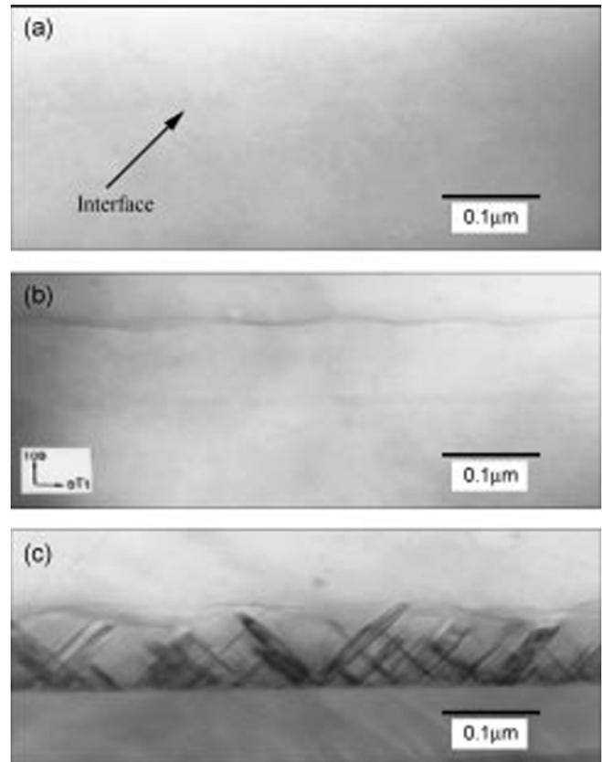
**Fig. 4.** (a) XTEM micrograph of the epitaxial film (Sample 8), which is blow-dried without water rinsing. (b) XTEM micrograph of the epitaxial film (Sample 9), in which the rinsing and blow drying steps are removed. (c) XTEM micrograph of the epitaxial film (Sample 10), in which the rinsing and blow drying steps are removed and the wafer is kept for several hours in a cleanroom before loading into the load lock chamber.
