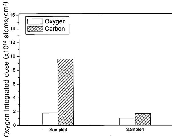
**Fig. 2.** Interfacial oxygen and carbon concentration based on SIMS data. Sample 3 is rinsed in DI water and then spun-dried, while sample 4 is spun-dried without rinsing. Both samples are *in situ* cleaned at 660°C.
