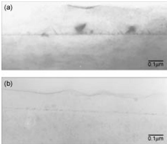
**Fig. 3.** Comparison of two samples cleaned with and without a rinsing step. They are blow-dried and do not experience an *in-situ* cleaning prior to epitaxial deposition at 600°C. (a) XTEM micrographs of sample 6 rinsed in DI water. (b) XTEM micrographs of sample 7, without rinsing. The structural quality of the epilayer/ substrate interface in the Sample without rinsing is higher than that of the Sample with rinsing.
