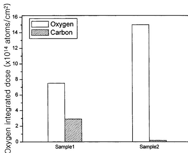
**Fig. 1.** Interfacial oxygen and carbon concentration based on SIMS data. Sample 2 is rinsed in DI water and then spin-dried, while sample 1 is spin-dried without rinsing. Both samples are *in-situ* cleaned at 600°C.
