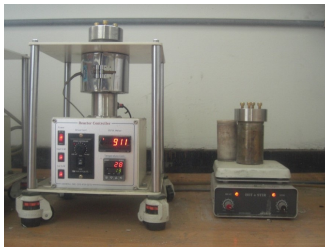
Fig. 1. Equipment used for hydrolysis and hydrothermal processes
