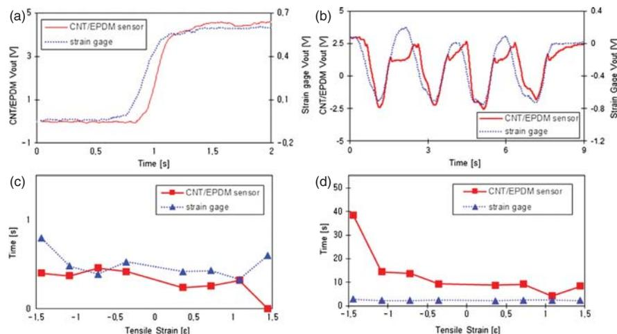
**Figure 5.** Voltage output responses of the CNT/EPDM (20 wt%) sensor system under deflections: (a) Static deflection test; (b) quasi-dynamic test with hand shaking; (c) rising time test; (d) settling time test.
