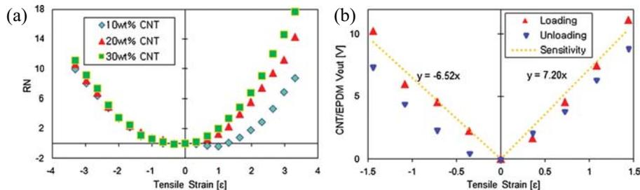
**Figure 3.** Strain sensing characteristics of the CNT/EPDM composite: (a) Piezoresistive property of the composites (10, 20, 30 wt%); (b) voltage output of the sensor (20 wt%) with hysteresis under static loading condition.
