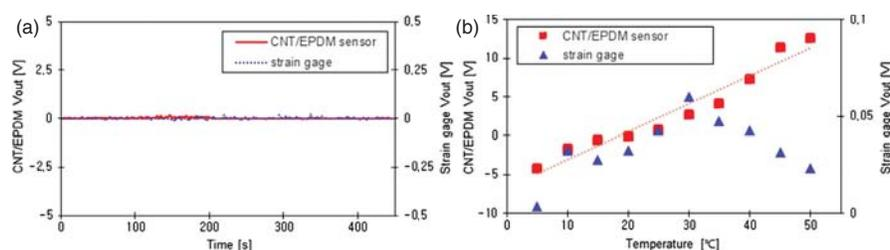
**Figure 4.** Voltage output responses of the CNT/EPDM (20 wt%) sensor system without load or deflection: (a) Drift test; (b) temperature test.
