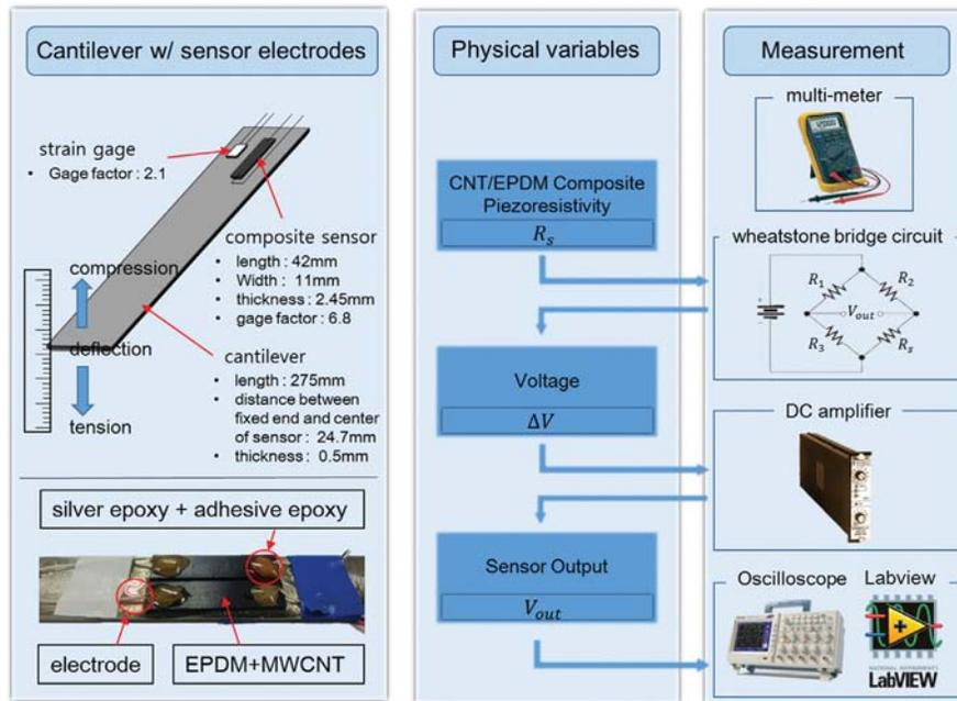
**Figure 2.** Schematic illustration of CNT-EPDM rubber composites to measure their piezoresistivity and sensing characteristics by using a signal processing with data acquisition system.
