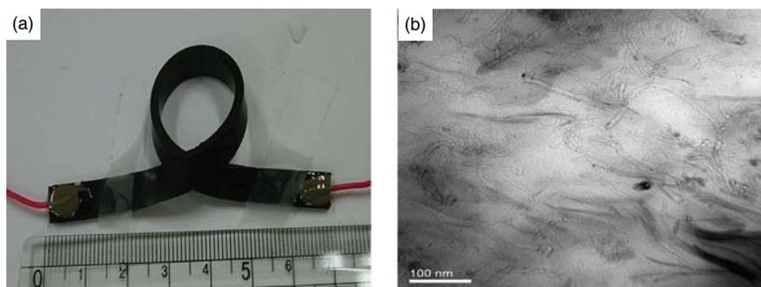
**Figure 1.** The CNT-EPDM rubber composite (10 wt%): (a) Flexible CNT/EPDM sensor electrode (150 mm × 5 mm × 2 mm, 160 k $\Omega$ ); (b) TEM image.
