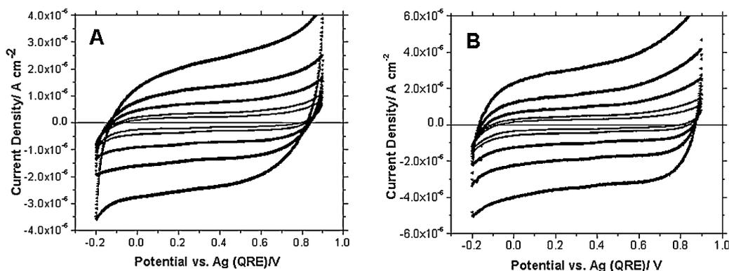
**Fig. 2.** Background cyclic voltammetric  $i$ - $E$  curves for a boron-doped diamond thin-film electrode as a function of the scan rate in (A) BMIMBF<sub>4</sub> and (B) 1 M KCl. Scan rates of 10, 20, 50, 100 and 200 mV s<sup>-1</sup> were employed. The BMIMBF<sub>4</sub> was purified by heating in vacuum (80 °C) overnight and storage over activated molecular sieves (5 Å).
