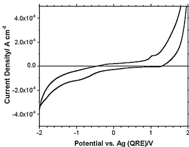
**Fig. 3.** Background cyclic voltammetric  $i$ - $E$  curve for a boron-doped diamond thin-film electrode in BMIMBF<sub>4</sub> showing the working potential window. Scan rate = 50 mV s<sup>-1</sup>. The BMIMBF<sub>4</sub> was purified by heating in vacuum (80 °C) overnight and storage over activated molecular sieves (5 Å).
