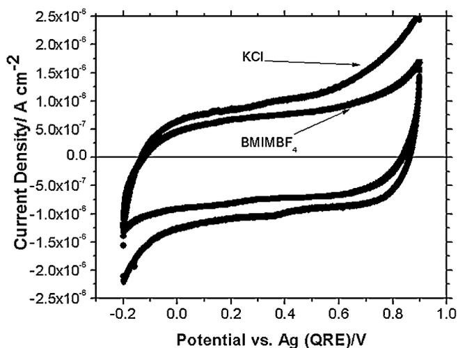
**Fig. 1.** Comparison of background cyclic voltammetric  $i$ - $E$  curves for a boron-doped diamond thin-film electrode in 1 M KCl and BMIMBF<sub>4</sub> at  $50$  mV s<sup>-1</sup>. The BMIMBF<sub>4</sub> was purified by heating in vacuum ( $80$  °C) overnight and storage over activated molecular sieves ( $5$  Å).
