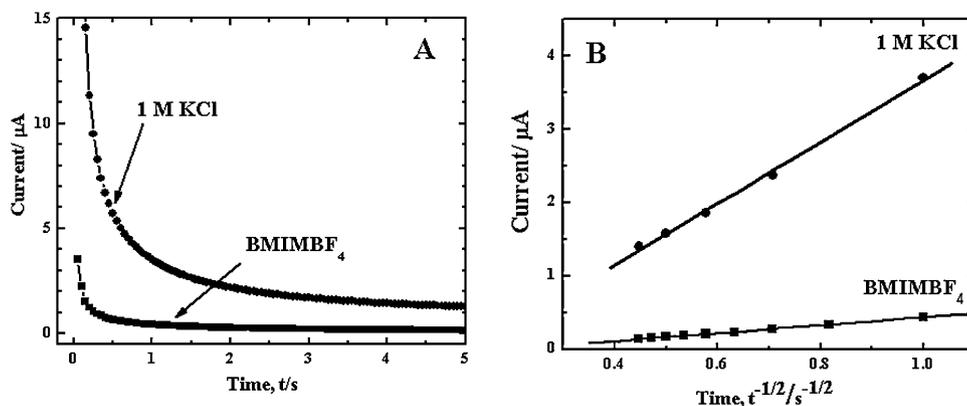
**Fig. 4.** (A) Chronoamperometric  $i-t$  profiles for the diffusion-limited oxidation of 0.1 mM FCA in 1 M KCl and BMIMBF<sub>4</sub>. The potential was stepped from 0 to 0.6 V vs. Ag/AgCl for KCl and from 0.3 to 0.9 V vs. Ag QRE for BMIMBF<sub>4</sub>. (B) Corresponding plots of  $i_j$  vs.  $t^{-1/2}$  calculated from current-time curves.  $i_j$  values were determined via background subtraction. The BMIMBF<sub>4</sub> was purified by storage over activated molecular sieves (5 Å).
