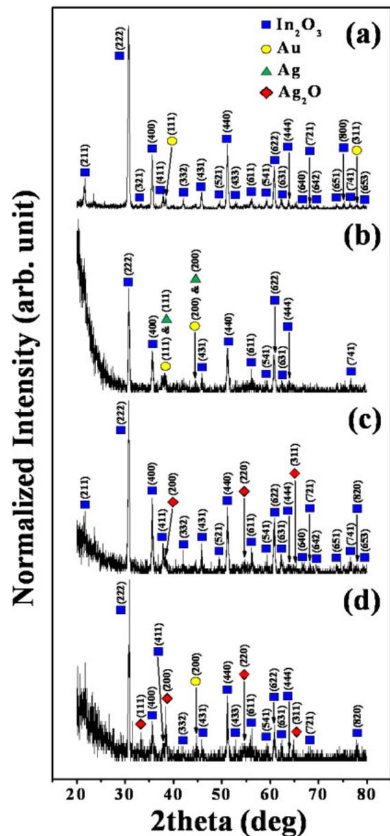
Fig. 1. (Color online) XRD patterns of (a) as-fabricated  $\text{In}_2\text{O}_3$  core nanowires, and  $\text{Ag}$ -coated core-shell nanowires (b) before and (c) after thermal annealing at  $500^\circ\text{C}$ .
