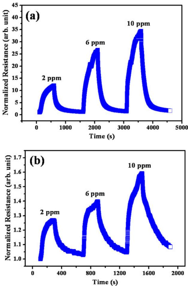
**Fig. 5.** (Color online) Typical dynamic response curve for various concentrations of NO<sub>2</sub> gas in a sensor fabricated from (a) as-fabricated In<sub>2</sub>O<sub>3</sub> core nanowires and (b) 500 °C-annealed In<sub>2</sub>O<sub>3</sub>/Ag core-shell nanowire.
