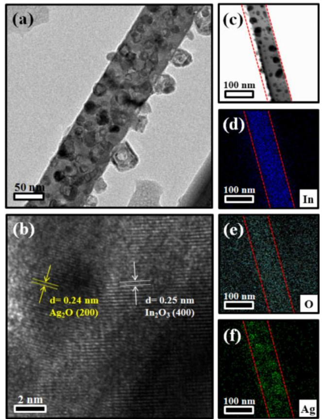
**Fig. 4.** (Color online) (a) Low-magnification TEM image of as-fabricated  $\text{In}_2\text{O}_3$  core nanowire. (b) Lattice-resolved TEM image, showing the  $\text{In}_2\text{O}_3$  core and nanoparticles. (c) TEM image of a typical nanowire, and EDX elemental maps of (d) In, (e) O, and (f) Ag elements.
