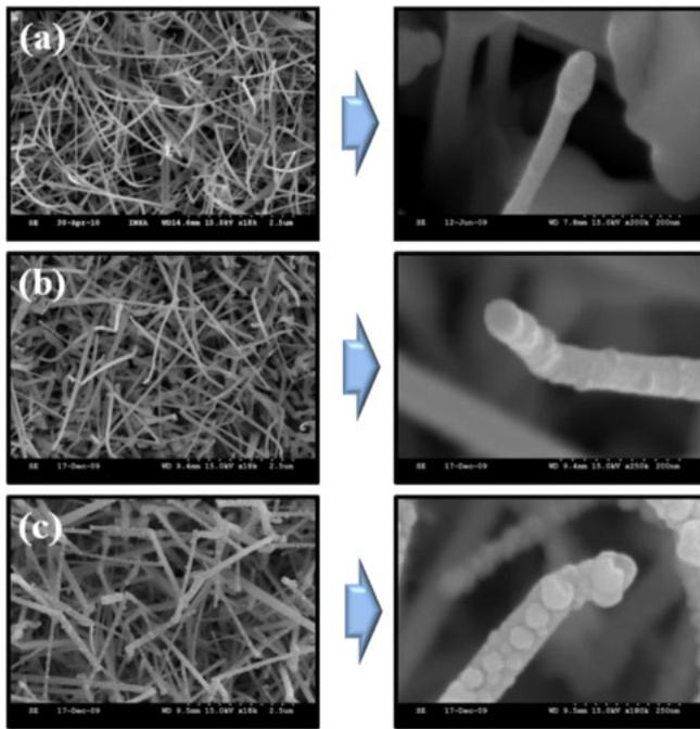
**Fig. 2.** (Color online) SEM images of (a) as-fabricated  $\text{In}_2\text{O}_3$  core nanowires, and Ag-coated core-shell nanowires (b) before and (c) after thermal annealing at 500 °C. Right-hand-side images correspond to the enlarged SEM images.
