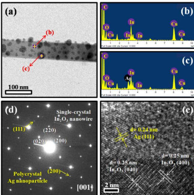
**Fig. 3.** (Color online) (a) Low-magnification TEM image of an as-fabricated  $\text{In}_2\text{O}_3$  core nanowire. EDX spectra of the (b) core and (c) nanoparticle regions indicated in (a). (d) SAED pattern and (e) lattice-resolved TEM image of enlarged area including the interface between  $\text{In}_2\text{O}_3$  core and nanoparticle.
