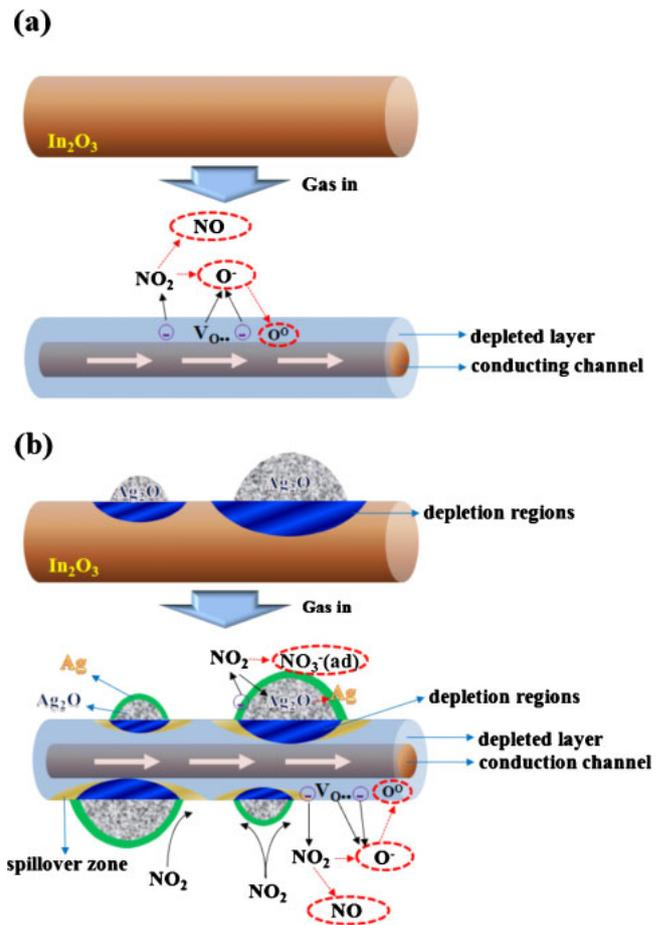
**Fig. 6.** (Color online) Schematics explaining the changes in the NO<sub>2</sub> sensing behavior (a) without and (b) with Ag<sub>2</sub>O functionalization.
