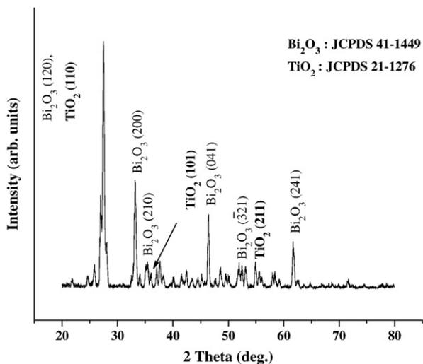
Fig. 3. XRD pattern of the  $\text{Bi}_2\text{O}_3$ -core/ $\text{TiO}_2$ -shell nanorods synthesized on (0001)  $\text{Al}_2\text{O}_3$ .
