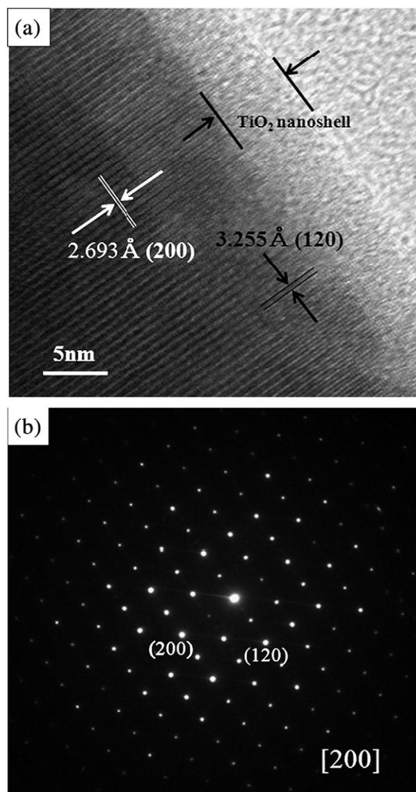
Fig. 2. (a) HRTEM image of a typical Bi<sub>2</sub>O<sub>3</sub> nanorod and (b) associated SAED pattern.
