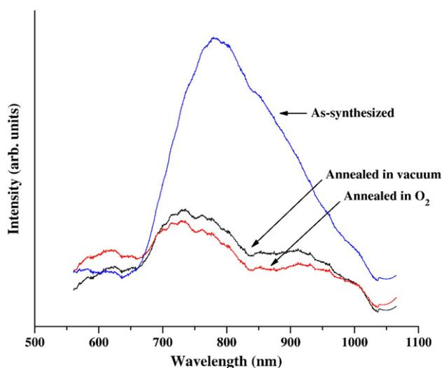
Fig. 5. Photoluminescence spectra of the  $\text{Bi}_2\text{O}_3$ -core/ $\text{TiO}_2$ -shell nanorods as-prepared and annealed.
