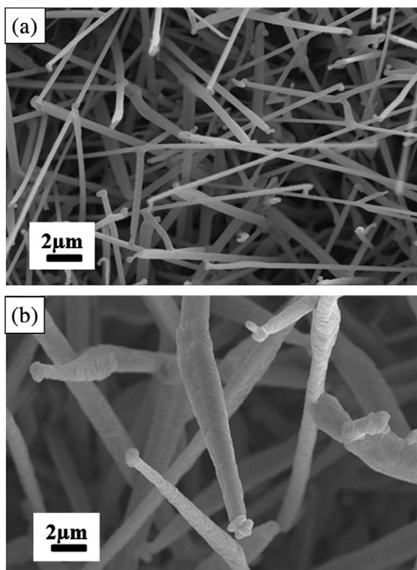
Fig. 1. SEM images of (a) Bi<sub>2</sub>O<sub>3</sub> nanorods synthesized by thermal evaporation of Bi powders on Al<sub>2</sub>O<sub>3</sub> substrates and (b) the Bi<sub>2</sub>O<sub>3</sub>-core/TiO<sub>2</sub>-shell nanorods prepared by coating the Bi<sub>2</sub>O<sub>3</sub> nanorods with TiO<sub>2</sub> by MOCVD at 650 °C for 4 h.
