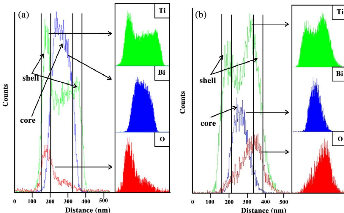
Fig. 6. EDX concentration profiles of Bi, Ti, and O along the diameter of a coaxial nanorod: (a) as-synthesized and (b) annealed in  $O_2$ .
