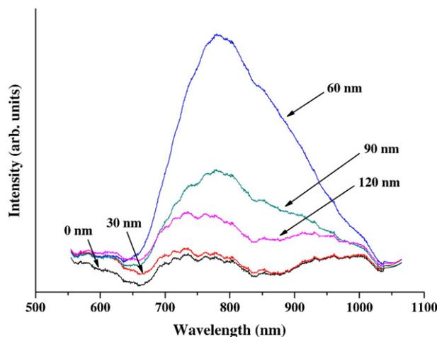
Fig. 4. Photoluminescence spectra of the  $\text{Bi}_2\text{O}_3$ -core/ $\text{TiO}_2$ -shell nanorods with different shell layer thicknesses.
