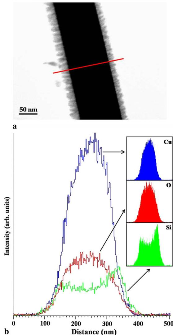
**Fig. 5** EDX concentration profiles of as-synthesized CuO-core/SiO<sub>x</sub>-shell nanowires
