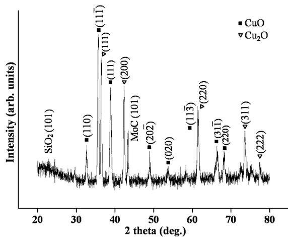
**Fig. 2** XRD patterns of CuO-core/SiO<sub>x</sub>-shell nanowires prepared by a two-step process: thermal oxidation of Cu foils at 600°C and sputter-deposition of SiO<sub>x</sub> at 100 W for 1 h
