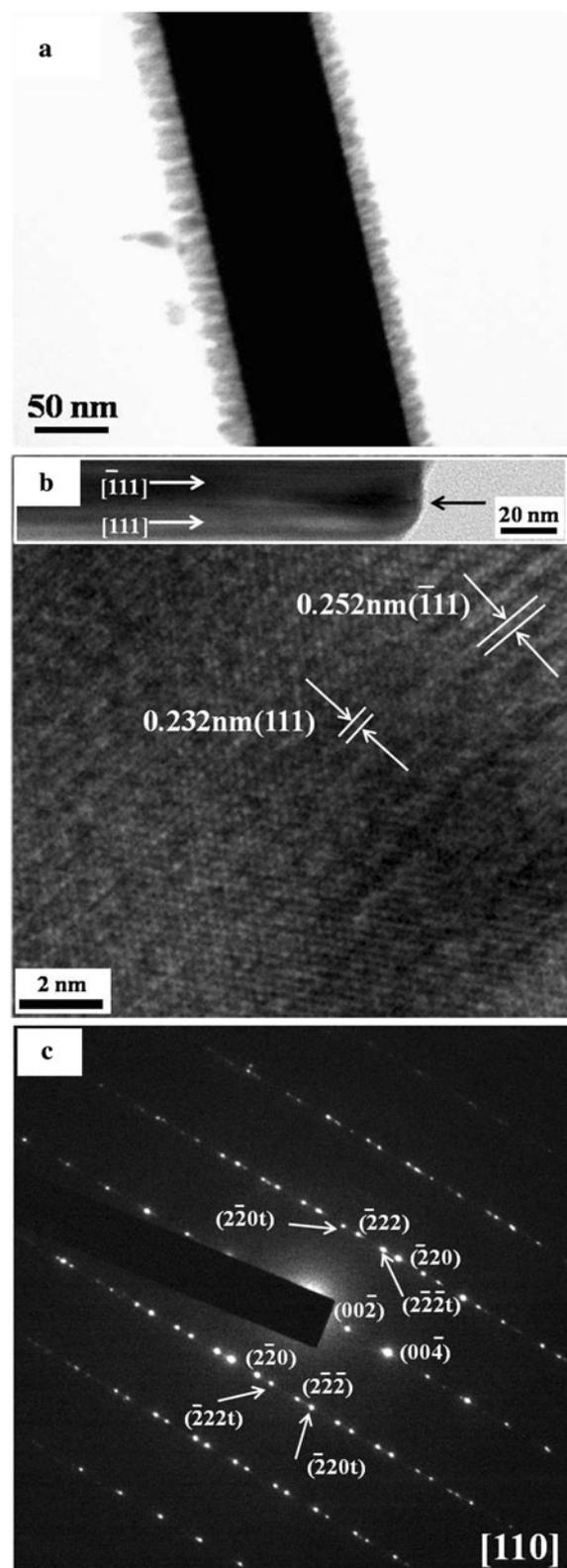
**Fig. 3** (a) Low-magnification TEM image of a typical CuO-core/SiO<sub>x</sub>-shell nanowire. (b) High-magnification TEM image of the nanowire. Indices without subscript *t* refer to the upperside of the nanowire shown in the inset, and indices with subscript *t* refer to the other side. The e-beam direction is parallel to the [110] axis. (c) The SAED pattern associated with the nanowire shown in (b)
