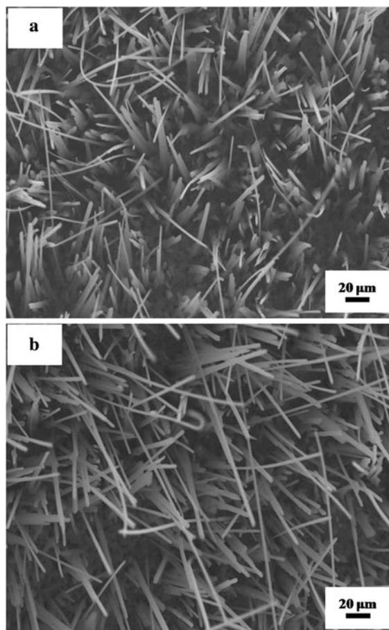
**Fig. 1** Top view SEM images of (a) CuO nanowires synthesized by thermal oxidation of Cu foils at 600°C for 5 h and (b)  $\text{SiO}_x$ -coated CuO nanowires
