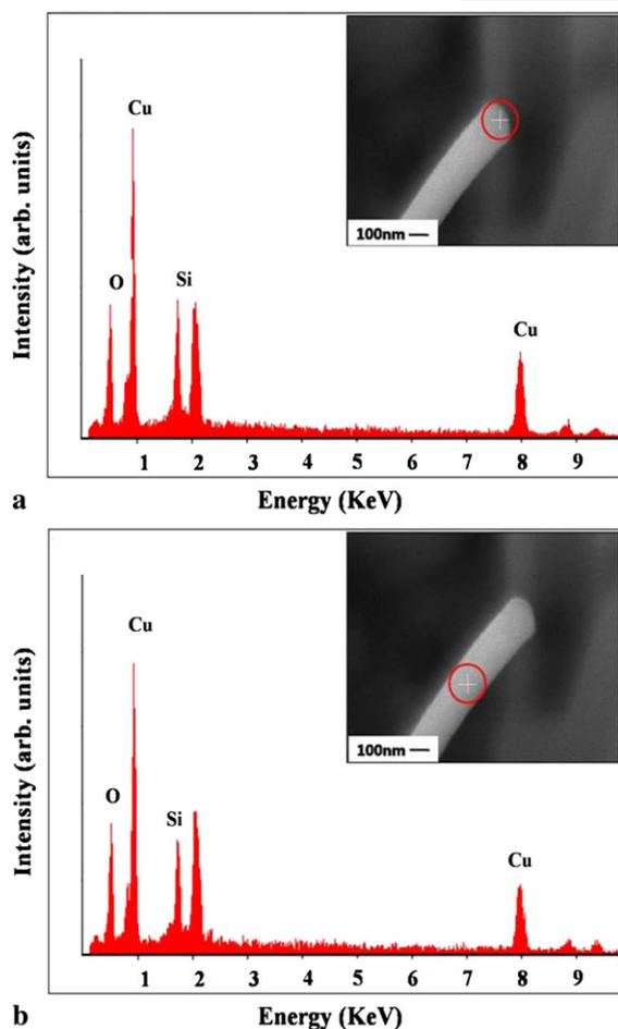
**Fig. 4** EDX spectra of a typical CuO-core/SiO<sub>x</sub>-shell nanowire synthesized by thermal oxidation of Cu foils and sputter-deposition of SiO<sub>x</sub>: (a) at the tip of the nanowire as shown as the area marked '+' in the SEM image of the inset and (b) in the middle of the nanowire as shown as the area marked '+' in the SEM image of the inset
