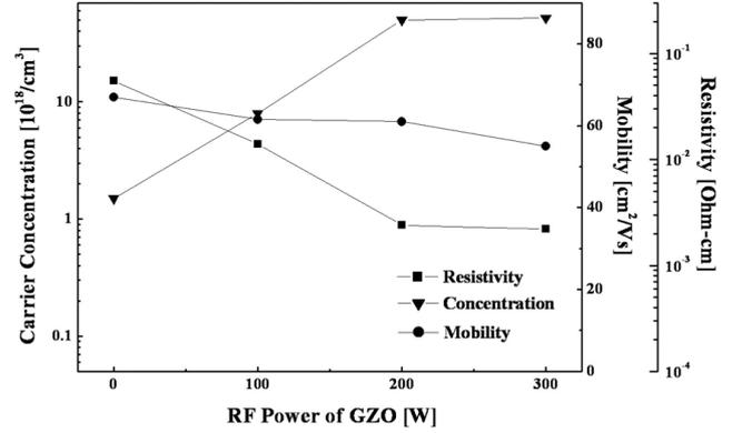
Fig. 1. Dependence of the carrier concentration, carrier mobility, and resistivity of AGZO thin films on the RF power for sputtering the GZO target. The DC power for sputtering the AZO target was fixed at 60 W.
