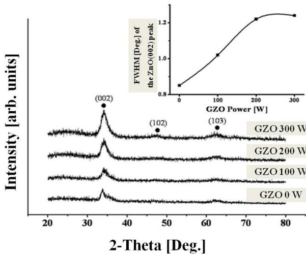
Fig. 2. X-ray diffraction patterns and FWHM of the ZnO (002) peak (inset) of AGZO thin films deposited by sputtering AZO and GZO targets simultaneously at different RF powers for GZO at a DC power of 60 W for AZO.
