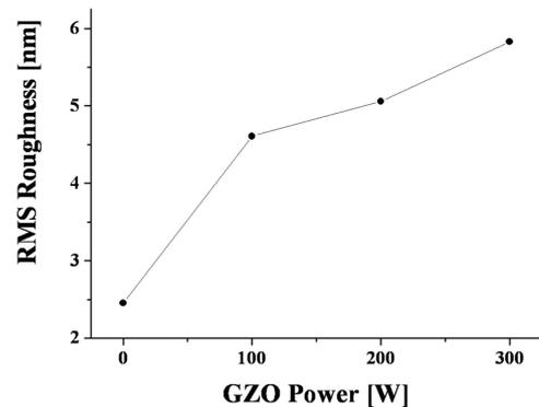
Fig. 4. RMS surface roughness of the AGZO thin film as a function of the RF power for sputtering the AZO target.
