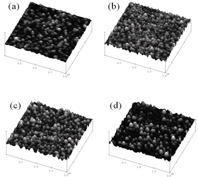
Fig. 3. AFM images of the surfaces of AGZO thin films deposited by sputtering AZO and GZO targets simultaneously at different RF powers for GZO and a DC power of 60 W for AZO.
