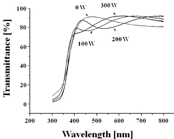
Fig. 5. Optical transmittance spectra for AGZO thin films deposited by cosputtering at different RF powers for GZO and a DC power of 60 W for AZO.
