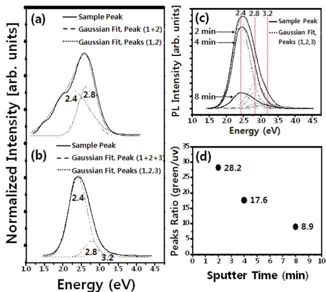
Fig. 3. Normalized PL spectra of (a) MgO core nanowires and (b) MgO/ZnO core-shell nanowires sputtered for 4 min. (c) Comparison of PL intensities of MgO/ZnO core-shell nanowires sputtered for 2, 4, and 8 min. (d) Variation of the green-to-UV peak intensity ratio for samples sputtered for 2, 4, and 8 min.
