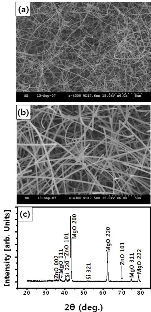
Fig. 1. SEM images of the MgO/ZnO core-shell nanowires sputtered for (a) 2 min and (b) 8 min. (c) XRD pattern of MgO/ZnO core-shell nanowires sputtered for 4 min.
