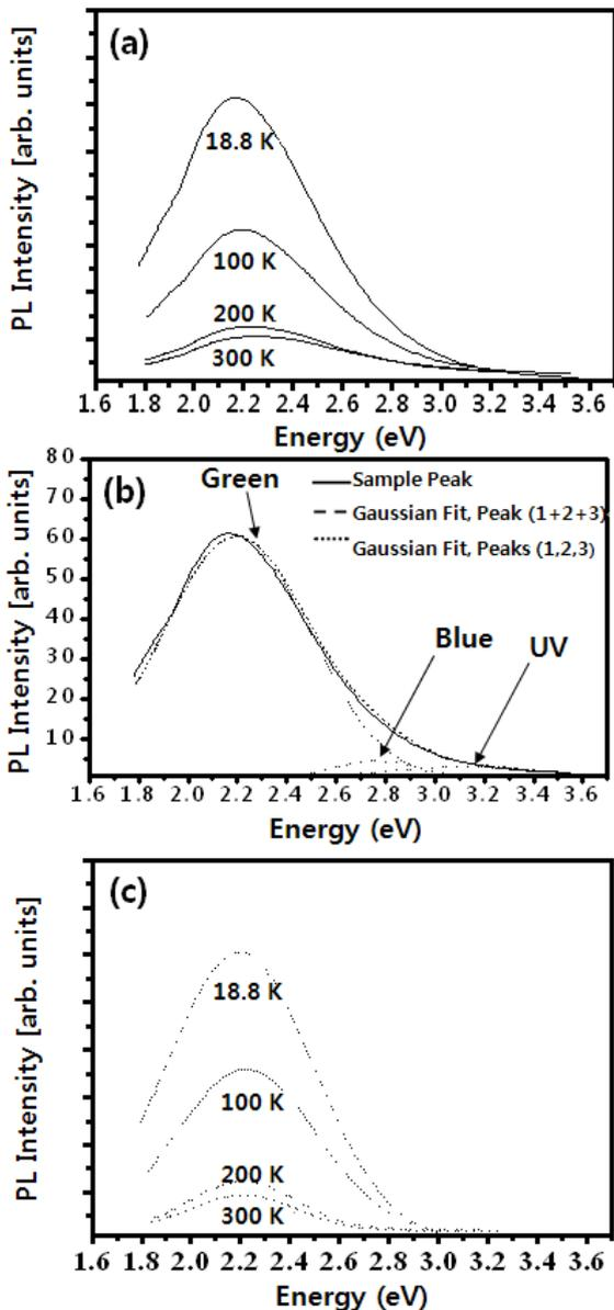
Fig. 4. (a) Temperature-dependent PL of MgO/ZnO core-shell nanowires sputtered for 8 min. (b) PL spectrum at 18.8 K with a Gaussian fitting analysis. (c) Variation of the green-emission bands (Gaussian functions) with varying measurement temperature.
