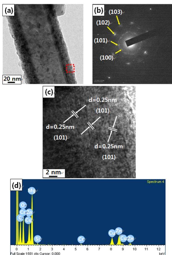
Fig. 2. (a) Representative TEM image of a MgO/ZnO core-shell nanowire sputtered for 4 min. (b) Corresponding SAED pattern. (c) Lattice-resolved TEM image enlarging the area enclosed by the dotted square in (a). (d) Corresponding TEM-EDX spectrum.
