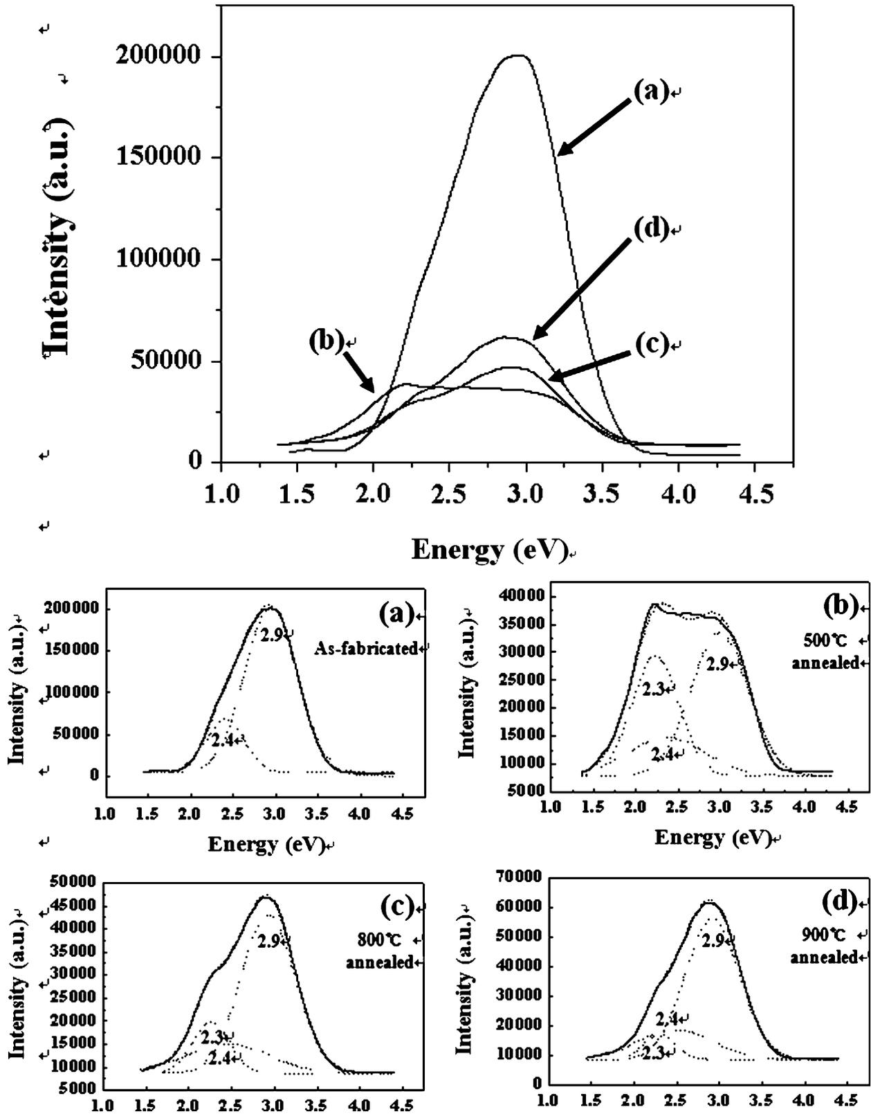
Fig. 4. PL spectrum of (a) as-fabricated  $\text{SiO}_x\text{-ZnO}$  core-shell nanowires and (b–d) annealed  $\text{SiO}_x\text{-ZnO}$  core-shell nanowires. The annealing temperature was set to (b) 500 °C, (c) 800 °C, and (d) 900 °C.
