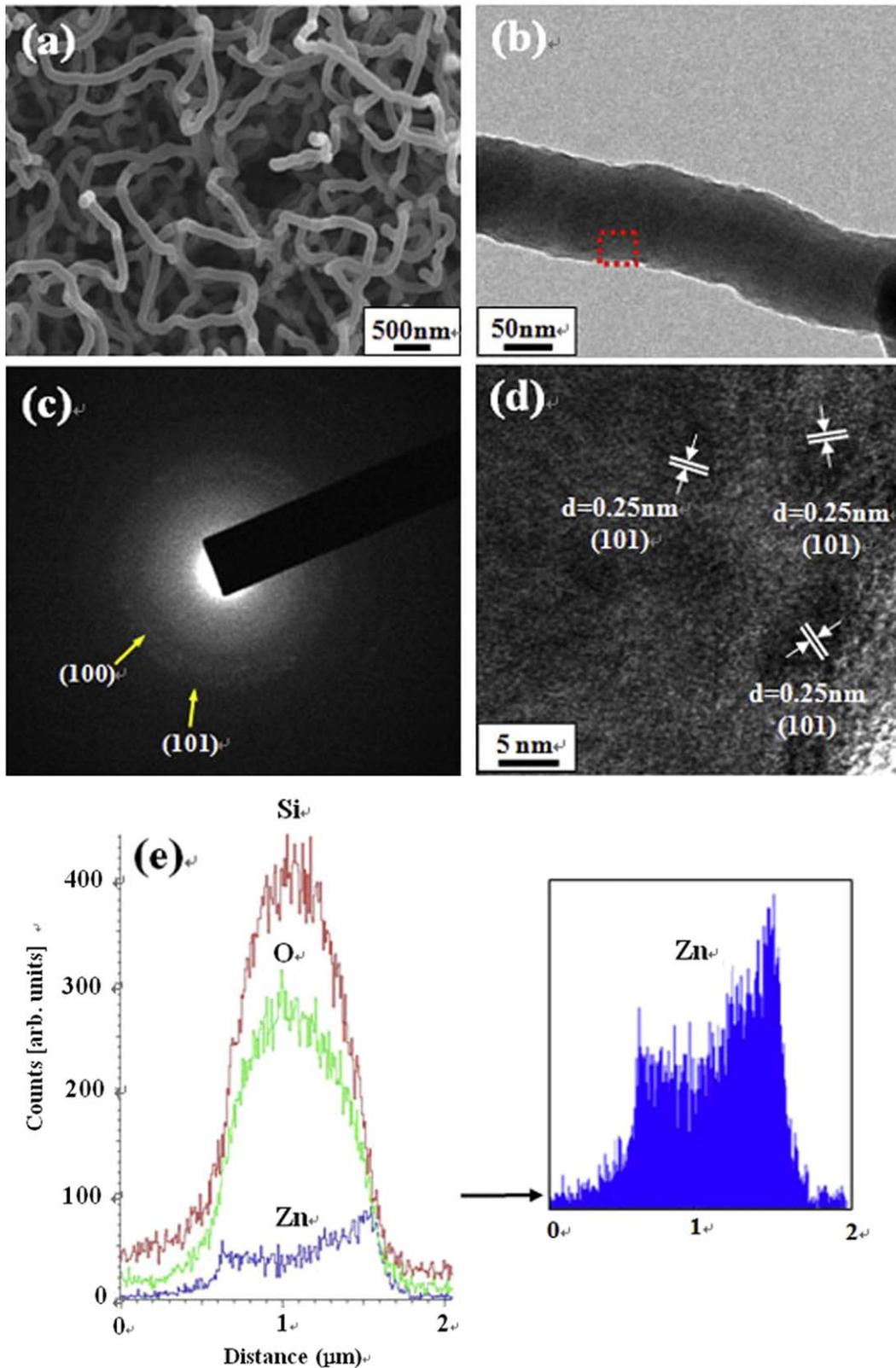
**Fig. 2.** (a) SEM and (b) TEM images of as-fabricated  $\text{SiO}_x\text{-ZnO}$  core-shell nanowires. (c) Corresponding selected area electron diffraction (SAED) pattern. (d) Enlarged TEM image from a marked area in (b). (e) TEM-EDX line concentration profiles for Si, O, and Zn, respectively, along the line drawing across the diameter of an as-fabricated  $\text{SiO}_x\text{-ZnO}$  core-shell nanowire.
