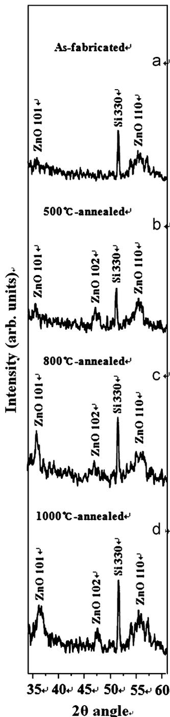
Fig. 1. XRD patterns of (a) as-fabricated  $\text{SiO}_x\text{-ZnO}$  core-shell nanowires and (b, c, and d)  $\text{SiO}_x\text{-ZnO}$  core-shell nanowires annealed at (b) 500 °C, (c) 800 °C, and (d) 1000 °C.
