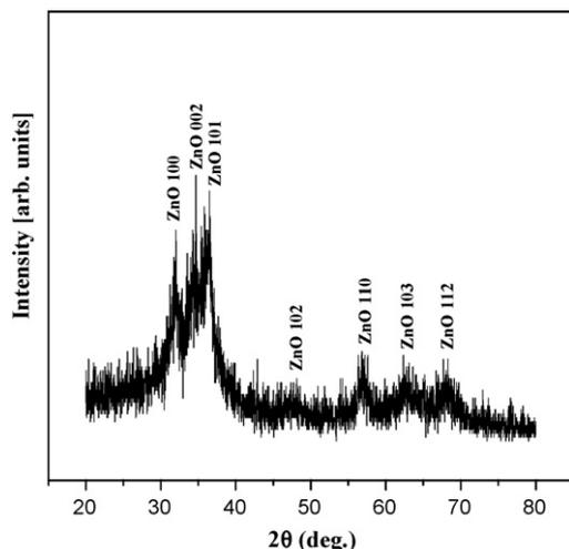
Fig. 4. XRD pattern of ZnO-coated Ga<sub>2</sub>O<sub>3</sub> nanowires with subsequent thermal annealing at 800 °C.
