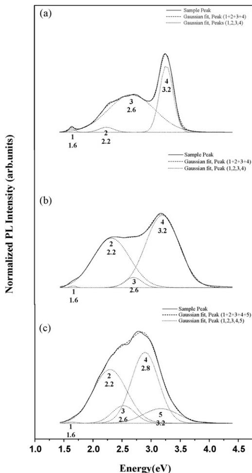
**Fig. 3.** Normalized PL spectra of (a) core  $\text{Ga}_2\text{O}_3$  nanowires, (b) ZnO-coated  $\text{Ga}_2\text{O}_3$  nanowires prior to thermal annealing, and (c) ZnO-coated  $\text{Ga}_2\text{O}_3$  nanowires after thermal annealing.
