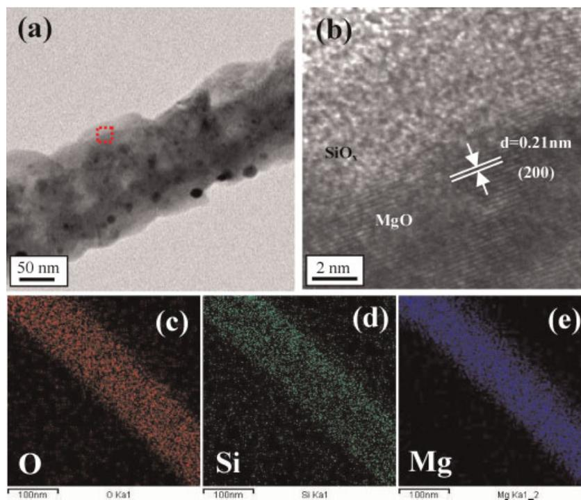
**Figure 4.** (a) TEM image of a MgO/SiO<sub>x</sub> core-shell nanowire after thermal annealing at 800°C. (b) Lattice-resolved TEM image enlarging a region enclosed by square box in (a). TEM elemental maps of (c) O, (d) Si, and (e) Mg concentrations from an annealed MgO/SiO<sub>x</sub> core-shell nanowire. This figure is available in color online at [www.interscience.wiley.com/journal/pat](http://www.interscience.wiley.com/journal/pat)
