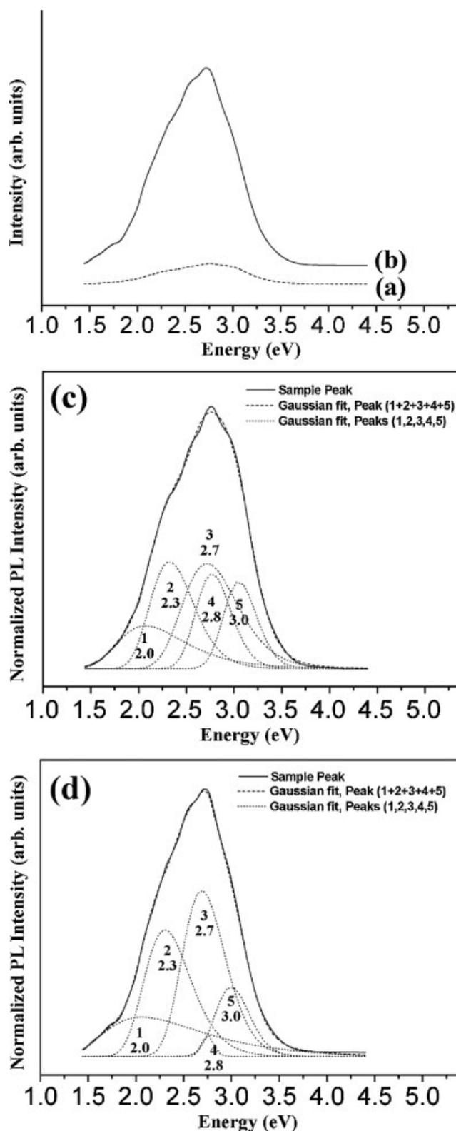
**Figure 5.** Room-temperature PL emission spectra of annealed MgO/SiO<sub>x</sub> core-shell nanowires with an annealing temperature of (a) 600°C and (b) 1000°C. Gaussian fitting analyses of (c) 600°C- and (d) 1000°C-annealed samples, indicating that both emission bands are superimposition of five emission peaks.
