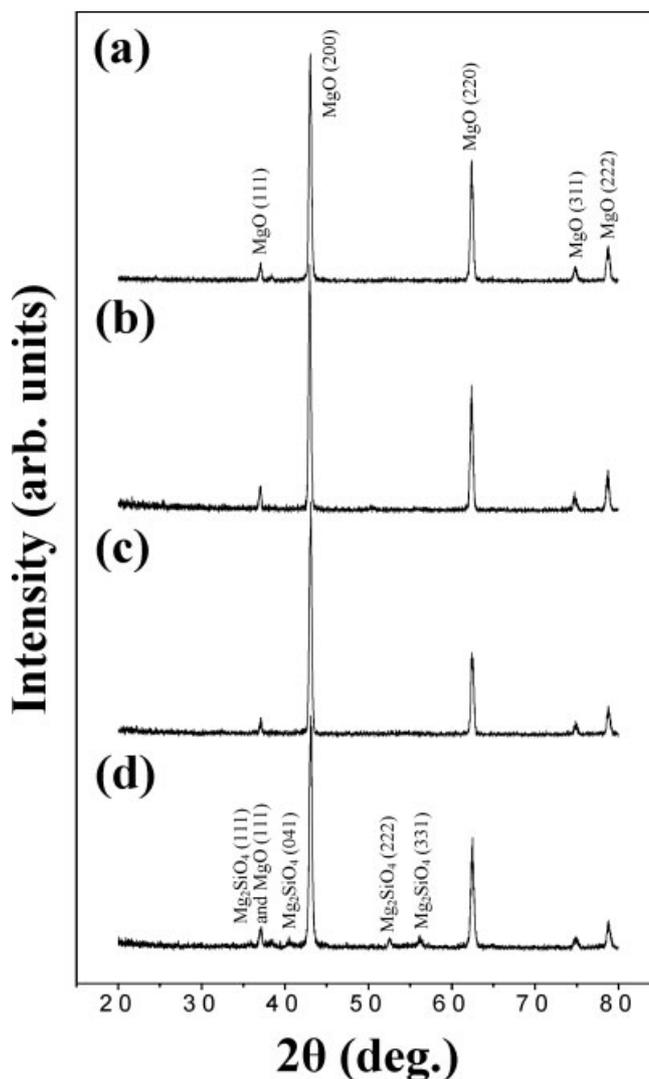
**Figure 2.** XRD patterns of (a) core  $\text{MgO}$  nanowires, (b) as-deposited core-shell nanowires, (c)  $600^\circ\text{C}$ -annealed core-shell nanowires, and (d)  $800^\circ\text{C}$ -annealed core-shell nanowires.
