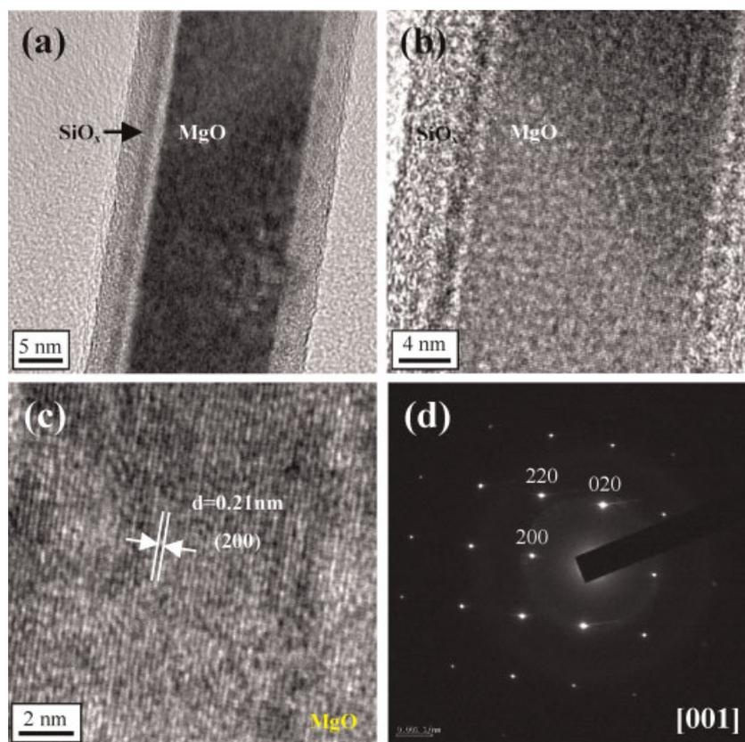
**Figure 3.** (a) TEM image of a MgO/SiO<sub>x</sub> core-shell nanowire prior to thermal annealing. (b) TEM image showing an enlargement of core and shell regions. (c) Lattice-resolved TEM image enlarging a core region in (b). (d) Corresponding SAED pattern. This figure is available in color online at [www.interscience.wiley.com/journal/pat](http://www.interscience.wiley.com/journal/pat)
