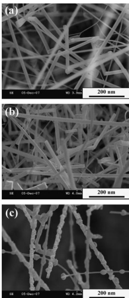
**Figure 1.** Top-view SEM images of (a) as-synthesized, (b)  $600^\circ\text{C}$ -annealed, and (c)  $800^\circ\text{C}$ -annealed  $\text{MgO}/\text{SiO}_x$  core-shell nanowires.
