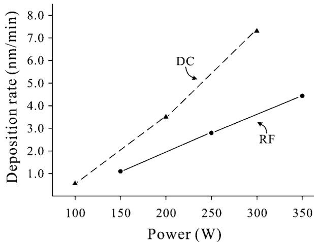
1 Variation of deposition rate of Cr film with sputtering power for rf and dc sputtering at constant pressure and constant substrate temperature
