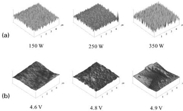
4 Images (AFM) of a Cr films deposited by rf magnetron sputtering at different rf powers and b electroplated Cr films deposited at different applied voltages
