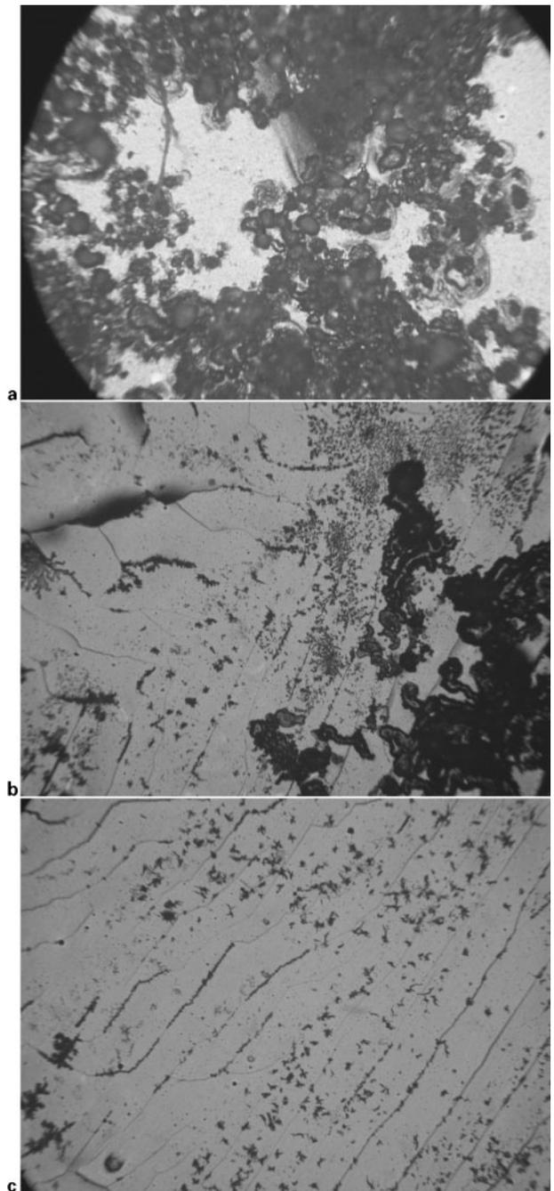
a electroplated Cr film; b Cr film deposited by dc sputtering; c Cr film deposited by rf sputtering
