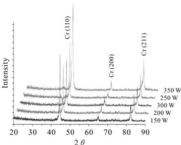
5 X-ray diffraction spectra for Cr films deposited by magnetron sputtering either dc or rf at different sputtering powers
