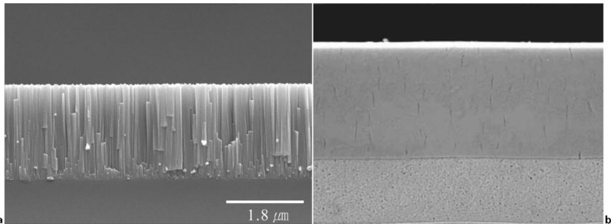
7 Cross-sectional SEM images of a sputter deposited and b electroplated Cr films
