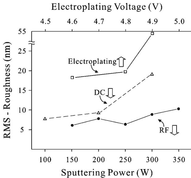
3 Variation of RMS surface roughness of Cr film with sputtering power for rf and dc sputtering at constant pressure and constant substrate temperature
