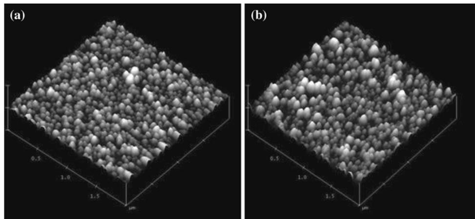
becomes rougher as the Al layer thickness is decreased. From the AFM images shown in Fig. 4a and b, it is evident that introduction of an Al interlayer makes the film surface smoother.
