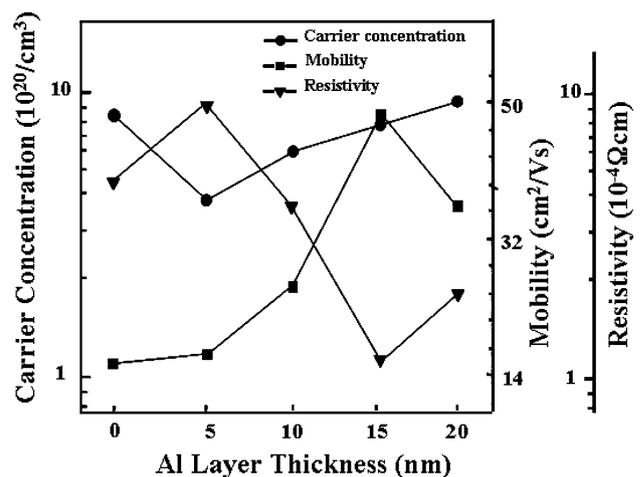
**Fig. 1** Dependence of the carrier concentration, the carrier mobility and the resistivity of the IZO/Al/GZO/ZnO multilayer film on the thickness of the Al interlayer
