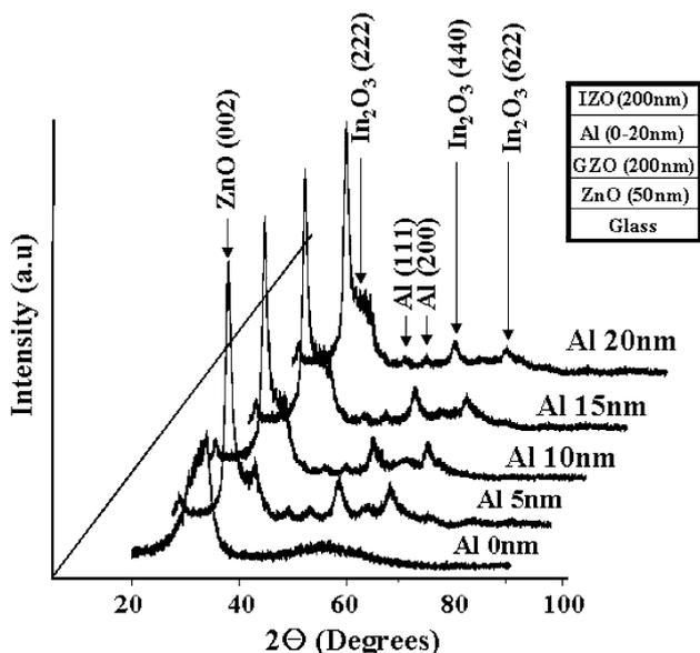
**Fig. 5** XRD patterns of IZO/Al/GZO/ZnO multilayer thin films with different Al interlayer thicknesses
