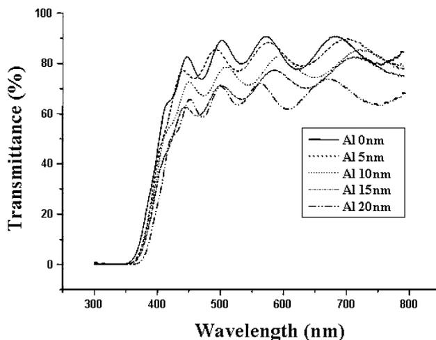
Fig. 2 Optical transmittance spectra for IZO/Al/GZO/ZnO multilayer thin films with different Al interlayer thicknesses
