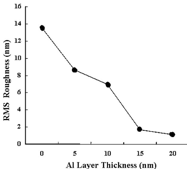
Fig. 3 The RMS surface roughness of the IZO/Al/GZO/ZnO multilayer thin film as a function of the Al interlayer thickness
