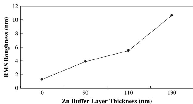
Fig. 3. Dependence of the RMS surface roughness of the ZnO thin film on the Zn buffer layer thickness.
