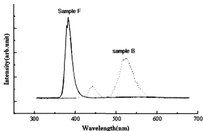
Fig. 4. PL spectra for ZnO thin films with and without a Zn buffer layer.
