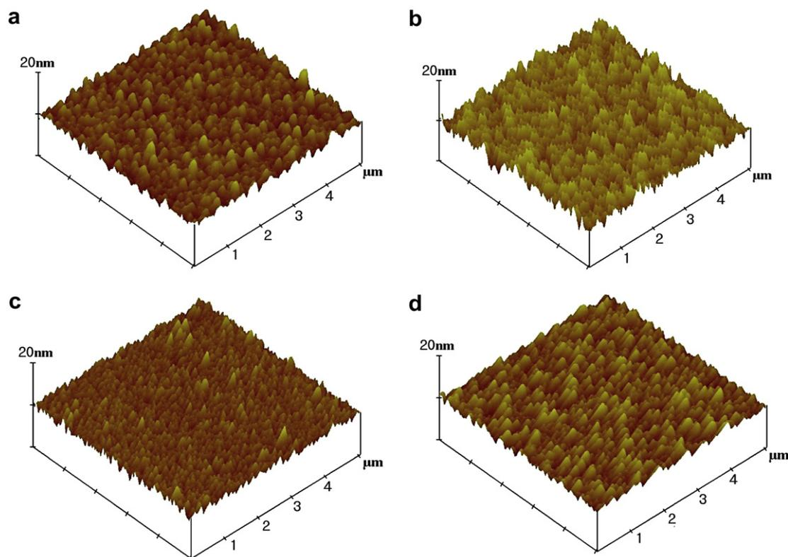
**Fig. 2.** AFM images of annealed ZnO/Zn/Si (100) samples with Zn buffer layers. (a) 0 nm, (b) 90 nm, (c) 110 nm, and (d) 130 nm thick.
