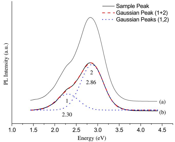
Fig. 5. PL spectra of uncoated (a) and ZnO-coated (b) MgO nanowires.
