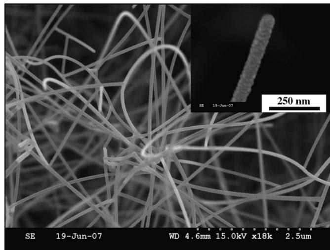
Fig. 2. SEM image of coated product (inset: typical closer-view SEM image of a ZnO-coated MgO nanowire).
