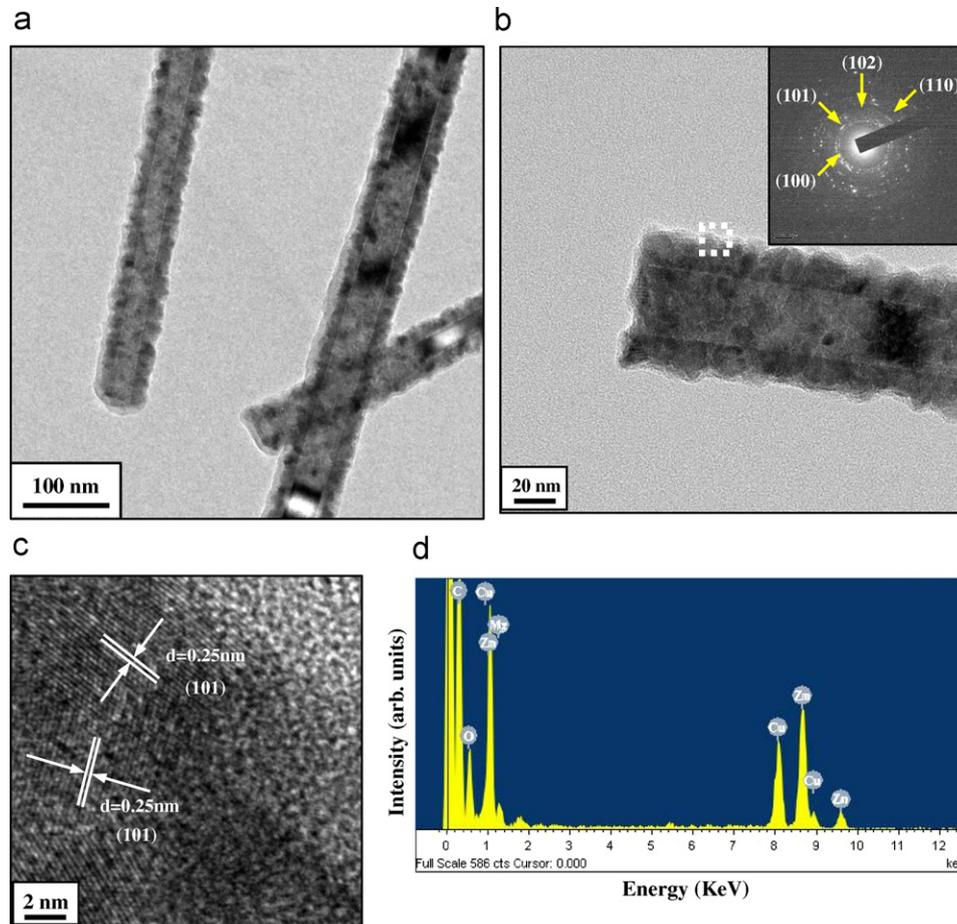
Fig. 3. (a) Low-magnification TEM image of coated product. (b) TEM image of a coated nanowire (inset: associated SAED pattern). (c) Lattice-resolved TEM image taken at the area marked with the dotted box in part (b). (d) Typical EDX spectrum from the coated nanowire.
