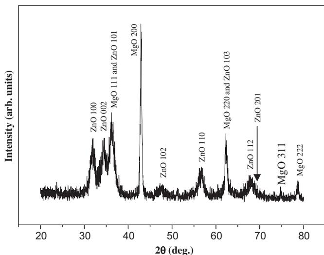
Fig. 1. XRD spectrum of the ZnO-coated MgO nanowires.
