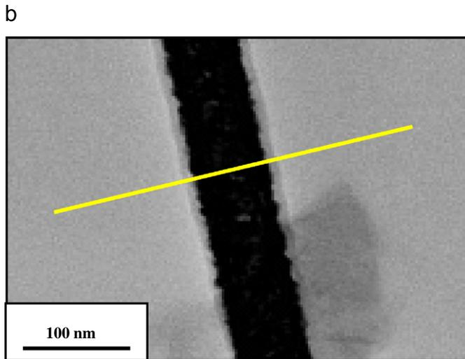
Fig. 4. EDX concentration profile of (a) Zn along the line drawing in a coated nanowire shown in part (b).
