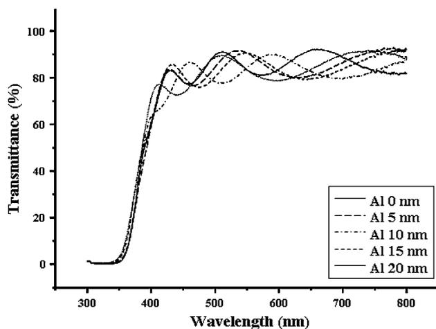
**Fig. 2** The optical transmittance of AZO/Al/ZnO/glass samples with different Al interlayer thicknesses in a wavelength range from 300 to 800 nm
