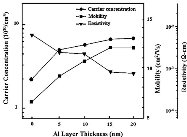
**Fig. 1** The carrier concentration, the carrier mobility, and the electrical resistivity of the AZO/Al/ZnO multilayer film as a function of the Al interlayer thickness
