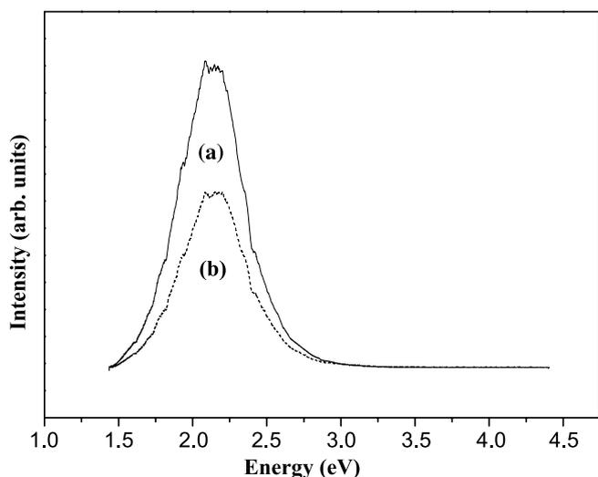
**FIGURE 6** PL spectrum of the products synthesized at (a) 850 °C and (b) 700 °C with a photoexcitation energy of 3.82 eV
