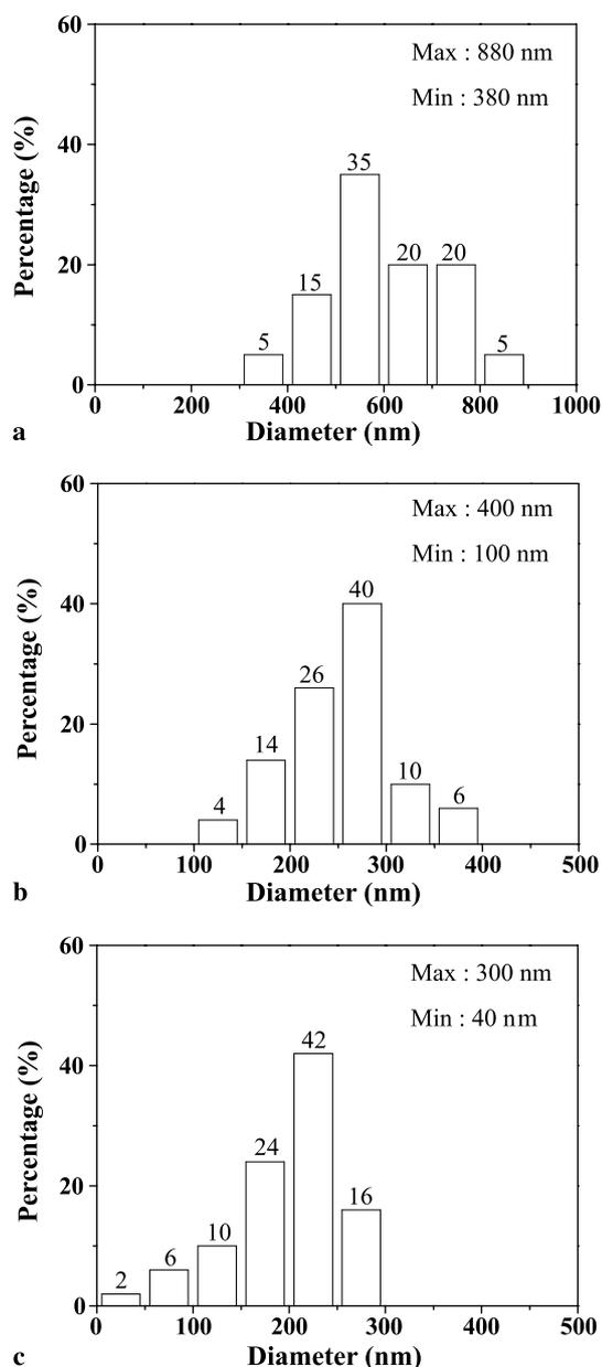
FIGURE 2 The diameter distribution of the products synthesized at (a) 850 °C, (b) 780 °C, and (c) 700 °C
