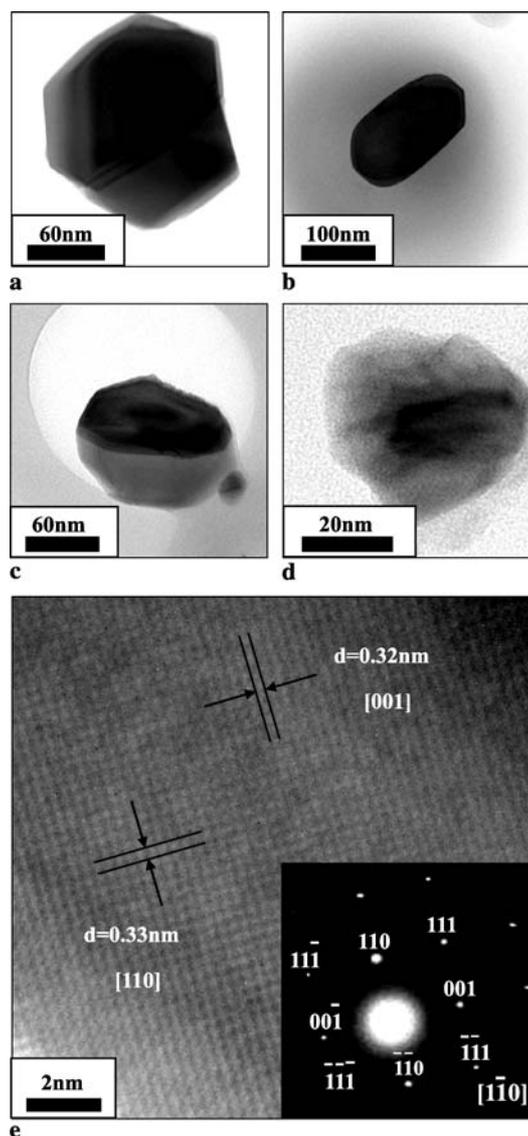
**FIGURE 5** (a)–(d) TEM images of the particles. (e) HRTEM image corresponding to an area in (c) (Inset: corresponding SAED pattern)
