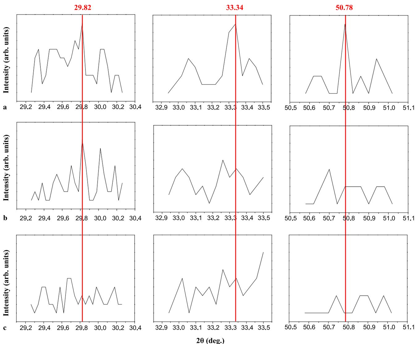
**FIGURE 4** Enlarged view of the XRD spectrum with the  $2\theta$  values in the range of  $29.3\text{--}30.2^\circ$ ,  $33.0\text{--}33.5^\circ$ , and  $50.6\text{--}51.0^\circ$ , from the samples synthesized at (a)  $850^\circ\text{C}$ , (b)  $780^\circ\text{C}$ , and (c)  $700^\circ\text{C}$
