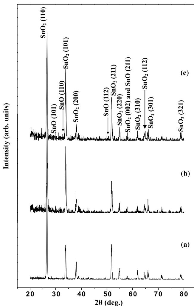
FIGURE 3 XRD pattern of the product synthesized at (a) 850 °C, (b) 780 °C, and (c) 700 °C
