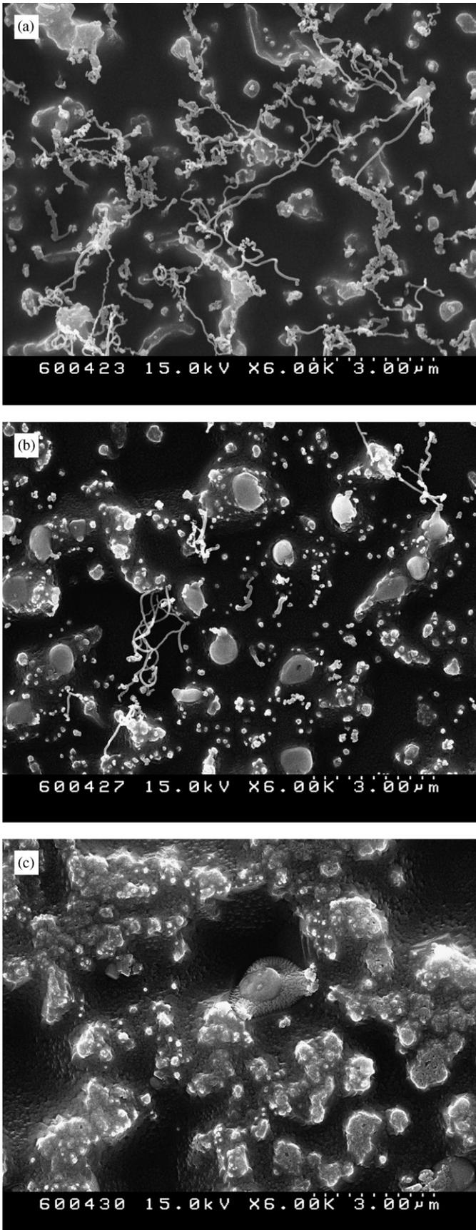
Fig. 3. Plan-view SEM images of the product with the Cu layer thicknesses of: (a) 15 nm; (b) 30 nm, and (c) 60 nm.
