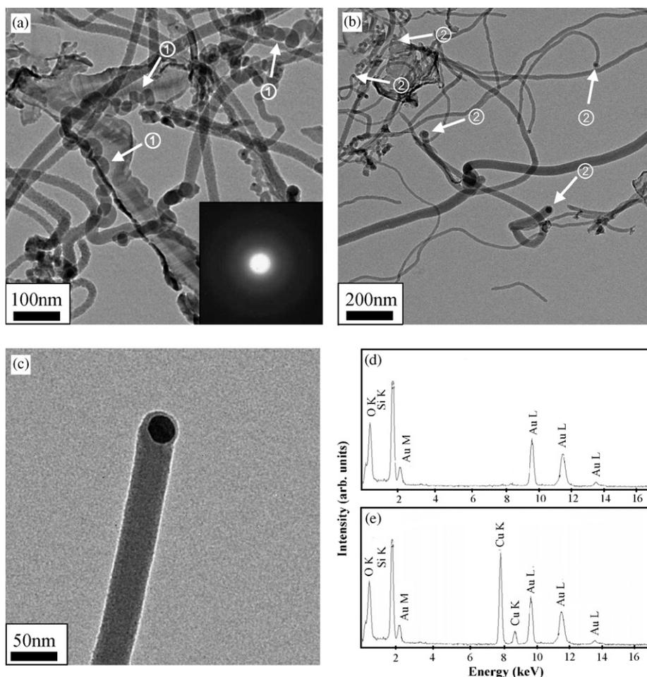
Fig. 2. (a,b) Low-magnification TEM images showing the general morphology of  $\text{SiO}_x$  nanowires (Arrow 1: helical nanowires or nanosprings; Arrow 2: nanoparticles). The lower right inset of (a) is the SAED pattern of  $\text{SiO}_x$  nanowires. (c) HRTEM image of a single nanowire. The nanowire terminates with a nanoparticle. EDX spectra of (d) the wire stem and (e) the wire tip.
