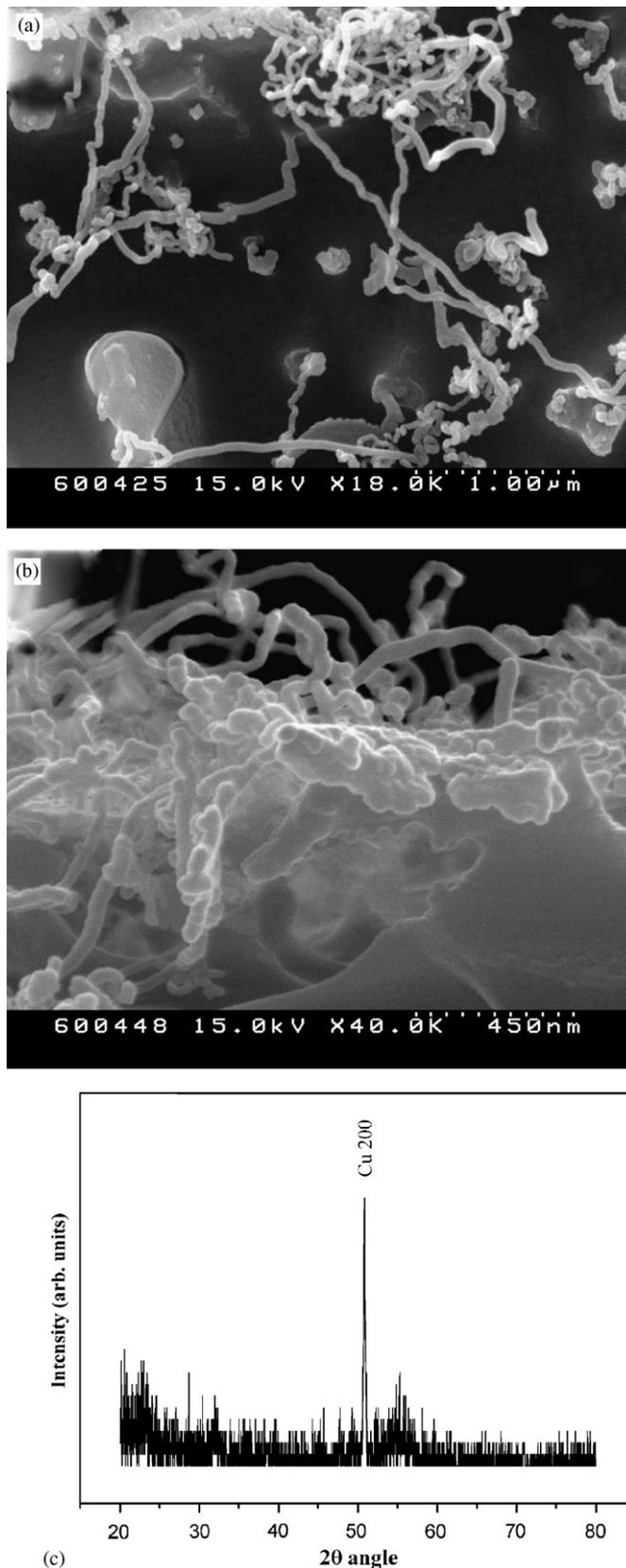
Fig. 1. (a) Plan-view; (b) side-view SEM images of the product and (c) X-ray diffraction pattern recorded from the product.
