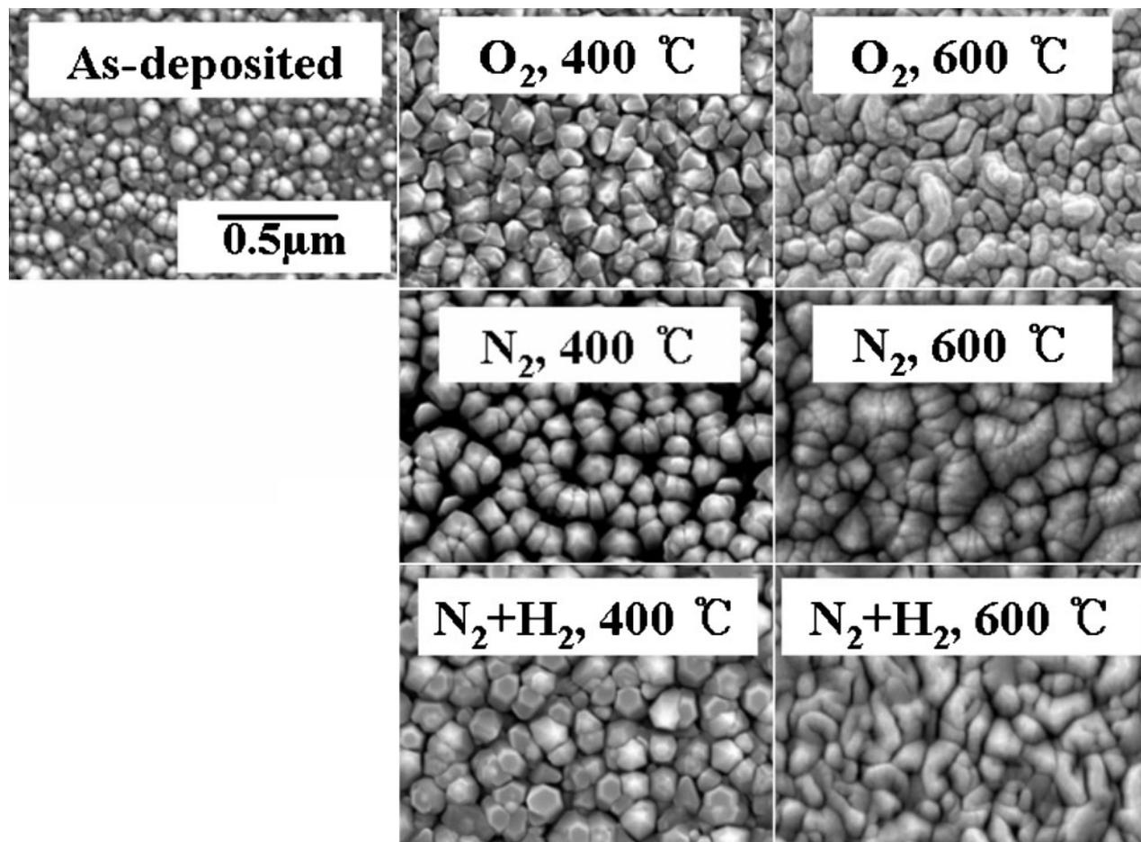
**2 Images (SEM) of GZO thin films annealed at different temperatures in different atmospheres**
