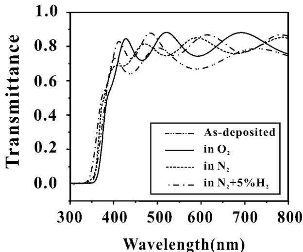
4 Optical transmittance spectra of GZO thin films as deposited and at 400°C annealed in different atmospheres
