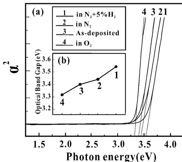
5 a plot of  $\alpha^2$  versus photon energy and b optical energy band gap values of GZO thin films annealed in different atmospheres, determined by extrapolation of the  $\alpha^2$  versus photo energy curve in Fig. 5a
