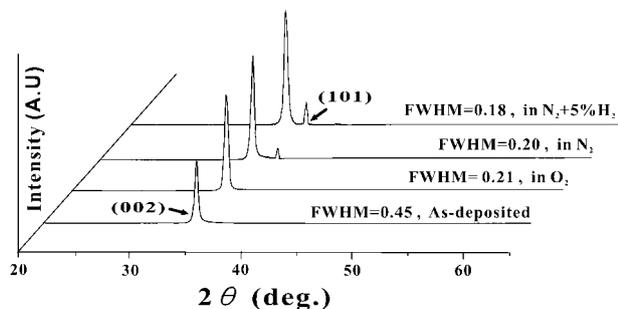
**1 X-ray diffraction spectra of GZO thin films annealed at 400°C in different atmospheres along with that of an as deposited GZO film**
