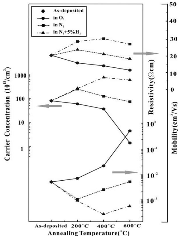
3 Electrical properties of GZO thin films as function of annealing temperature in different atmospheres
