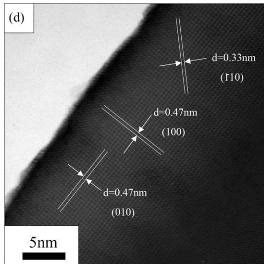
Fig. 3. (a) Low magnification TEM image of the products. (b) High magnification TEM image of a particle. (c) Corresponding SAED pattern. (d) HRTEM image corresponding to an area enclosed by the square in (b).
