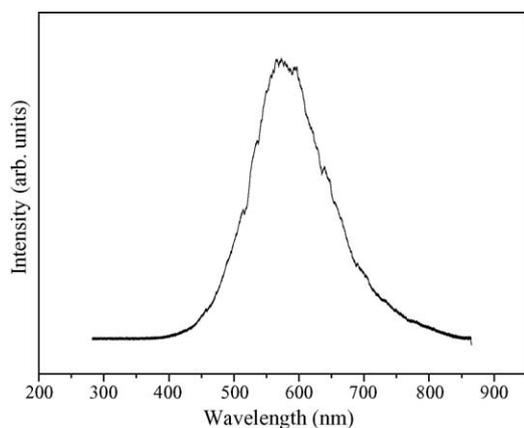
Fig. 4. Room temperature PL spectrum of the products with an excitation wavelength at 325 nm.
