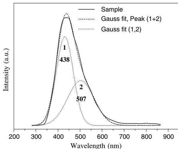
Fig. 5. Room-temperature PL spectrum of MgO nanowires with an excitation wavelength at 325 nm.
