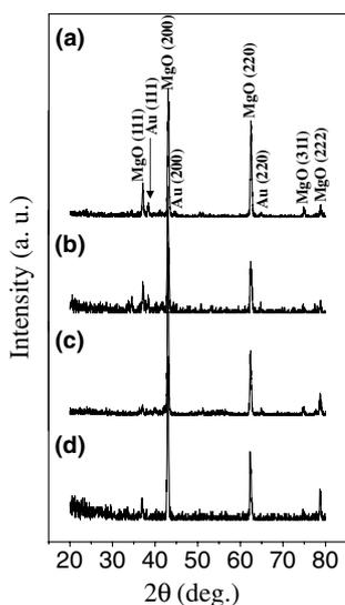
Fig. 2. XRD patterns recorded from the products: (a) without the predeposition annealing and with the predeposition annealing at (b) 300, (c) 500, and (d) 700 °C.
