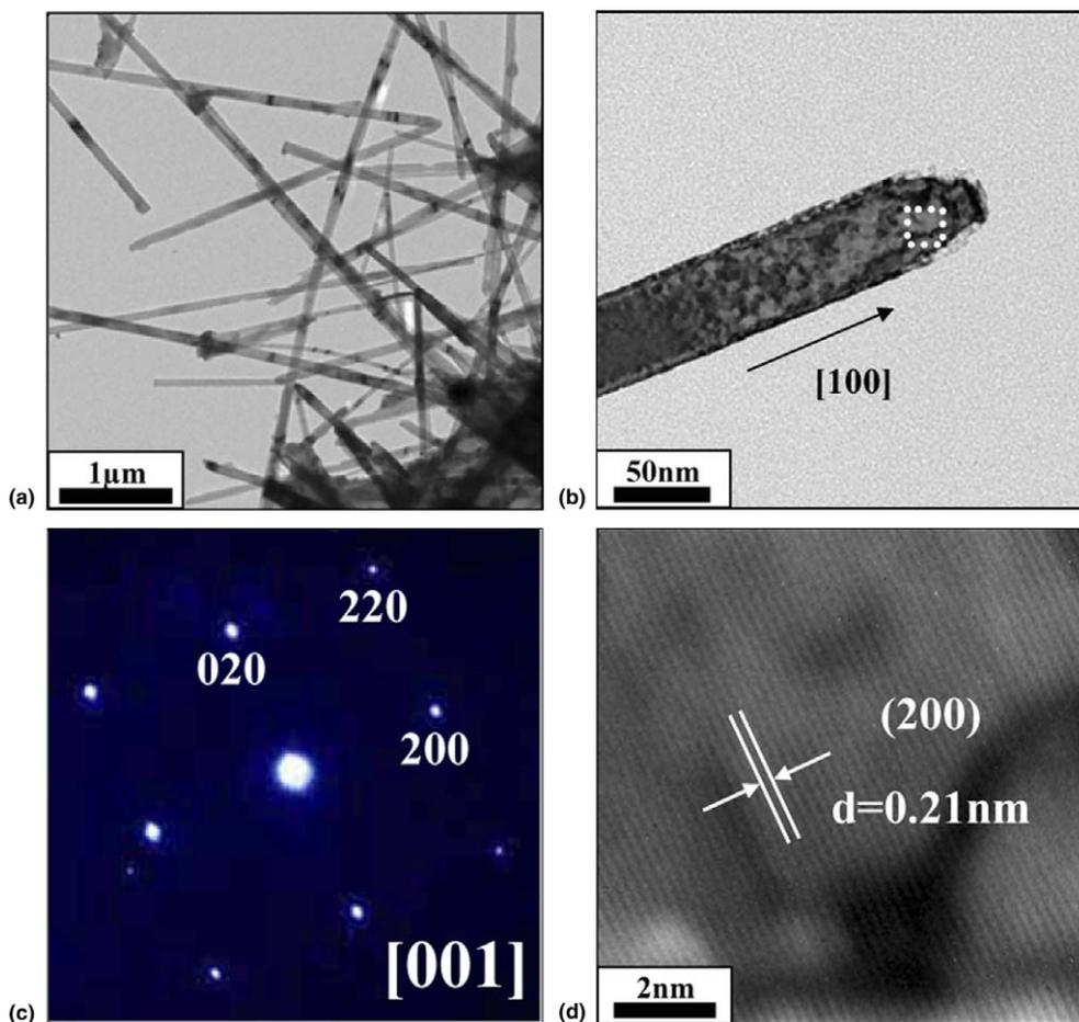
Fig. 4. (a) Low magnification TEM image of the product with the predeposition annealing at 700 °C. (b) TEM image of a single MgO nanowire. (c) Corresponding SAED pattern recorded along the [001] zone axis. (d) HRTEM image taken at the area marked with the dotted box in Fig. 4b.
