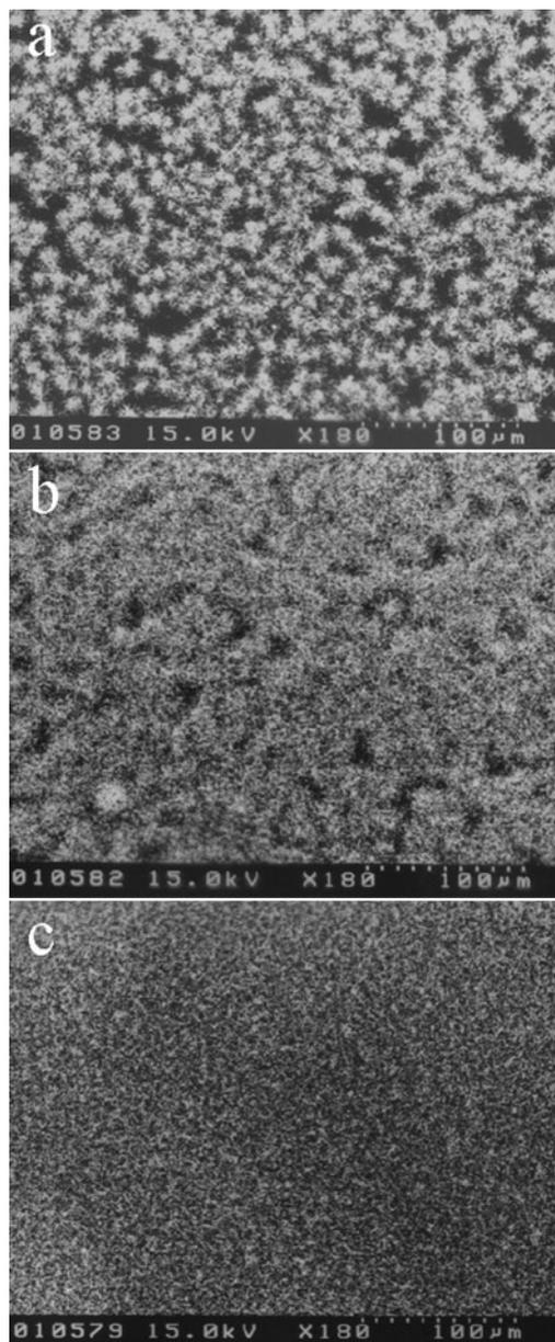
3 Cross-sectional SEM images of deposits on Si substrates with deposition times of *a* 3 min, *b* 4 min and *c* 5 min
