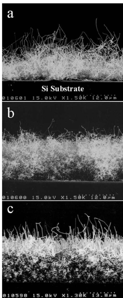
2 Plan view of SEM images of deposits on surface of Si substrate with deposition times of *a* 3 min, *b* 4 min and *c* 5 min
