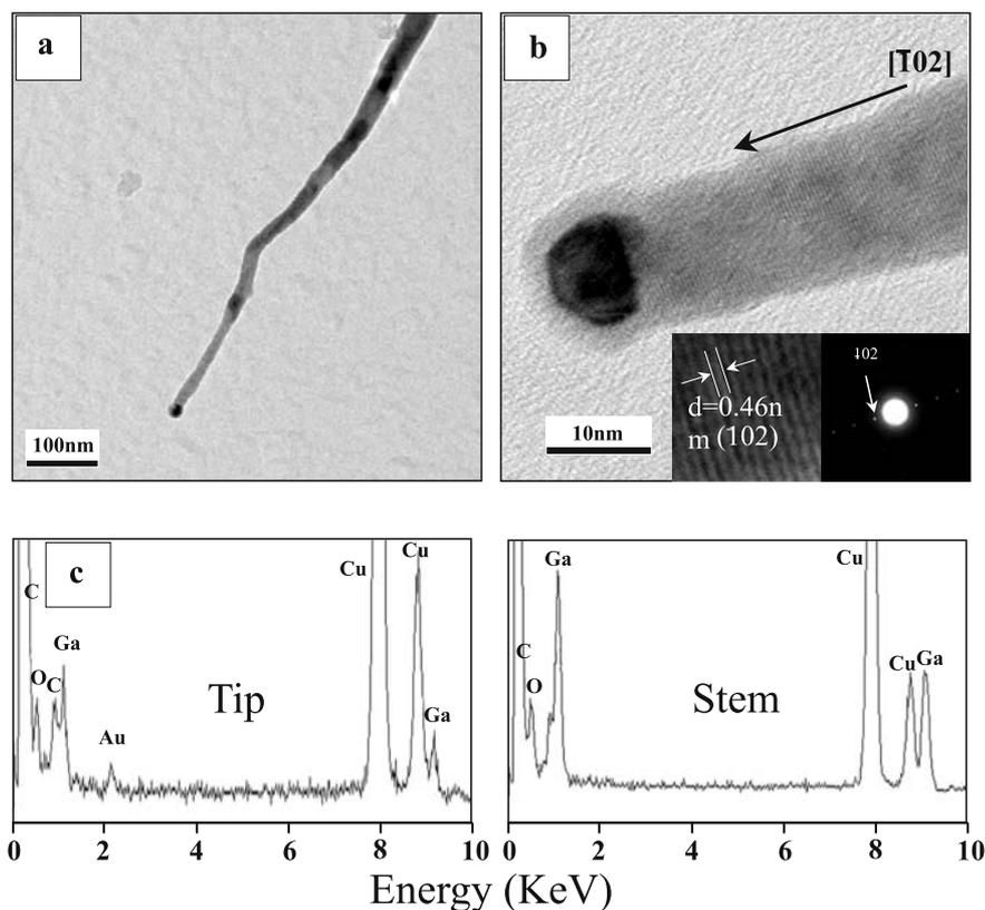
**FIGURE 3** a TEM and b HRTEM images of a single  $\beta$ -Ga<sub>2</sub>O<sub>3</sub> nanowire. The nanowire terminates with a nanoparticle. The magnified image and the corresponding electron-diffraction pattern are added in the *inset*. c EDS spectra of the wire tip and the wire stem
