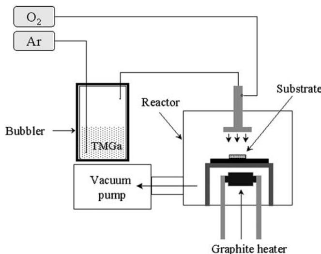
FIGURE 1 Schematic illustration of the MOCVD reactor
