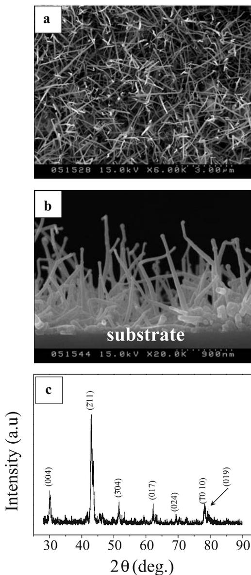
**FIGURE 2** a Plan-view and b side-view SEM images of the deposited nanowires. c X-ray diffraction patterns recorded from the  $\beta\text{-Ga}_2\text{O}_3$  nanowires
