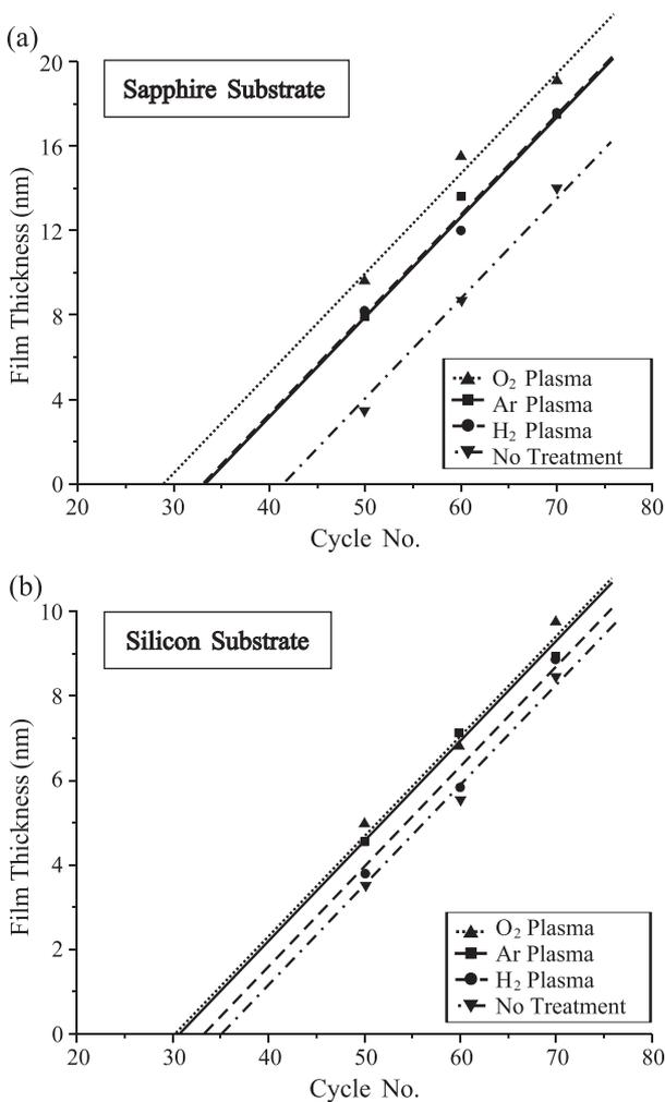
Fig. 3. Change of the thickness of the ZnO thin film deposited on (a) sapphire and (b) silicon substrates pretreated with different plasmas with ALE cycle number.
