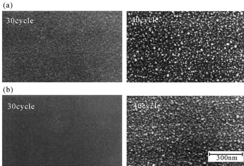
Fig. 2. Scanning electron micrographs of the ZnO thin films deposited on the sapphire substrate by ALE (a) with and (b) without O<sub>2</sub> plasma pretreatment for 30 and 40 cycles.
