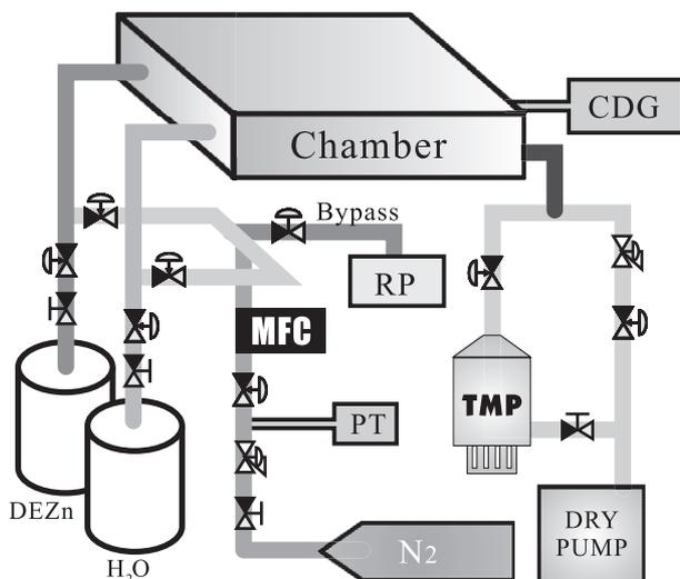
Fig. 1. A schematic of the ZnO ALE system.
