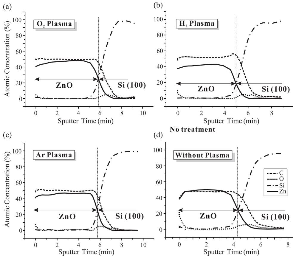
Fig. 5. AES depth profiles of ZnO thin films on the silicon substrate pretreated with (a) O<sub>2</sub> plasma, (b) H<sub>2</sub> plasma, (c) Ar plasma and (d) without plasma (cycle no. 50).
