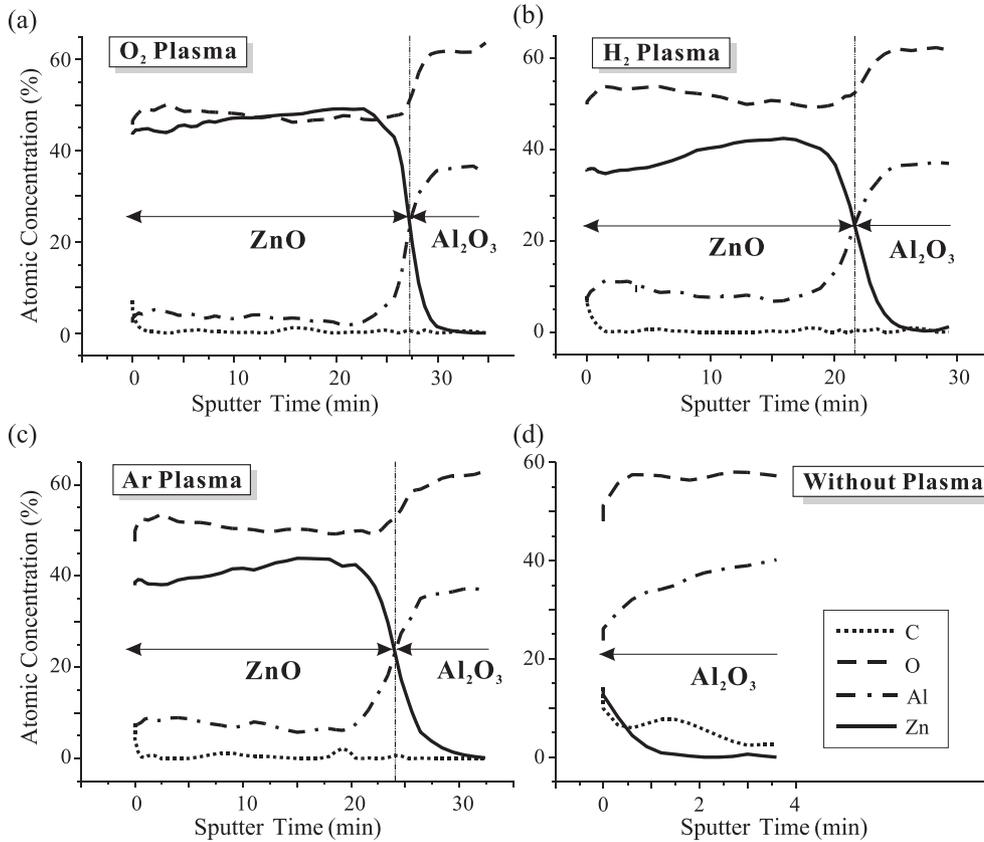
Fig. 4. AES depth profiles of ZnO thin films on the sapphire substrate pretreated with (a) O<sub>2</sub> plasma, (b) H<sub>2</sub> plasma, (c) Ar plasma and (d) without plasma (cycle no. 50).
