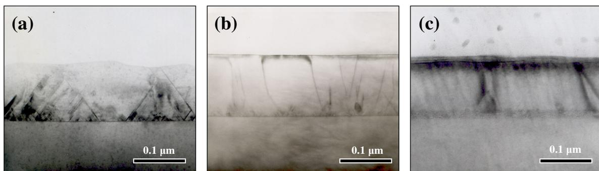
Fig. 2. Cross-sectional TEM images of Si films with (a) the microwave power of 150W, (b) the d.c. bias of +30V, and (c) with the cleaning time of 2 minutes.
