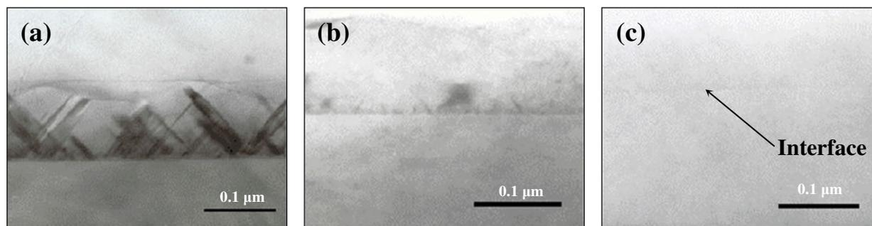
Fig. 1. Cross-sectional TEM images of Si films (a,b) without and (c) with the in-situ cleaning. The substrates were delivered to the deposition chamber (a) with several hours' air exposure and (b) with few seconds' air exposure after the ex-situ surface treatment.
