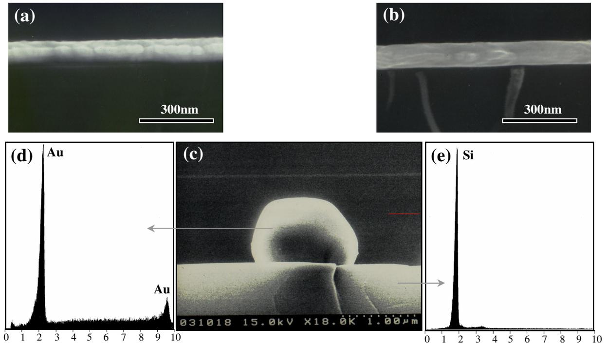
Fig. 1. Cross-sectional SEM images of Au thin films on Si substrate (a) without annealing, (b) with annealing at 400°C and (c) with annealing at 700°C. (d,e) EDX spectra of Au structure on Si
