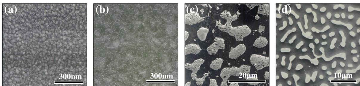
substrate with annealing at 700°C.
