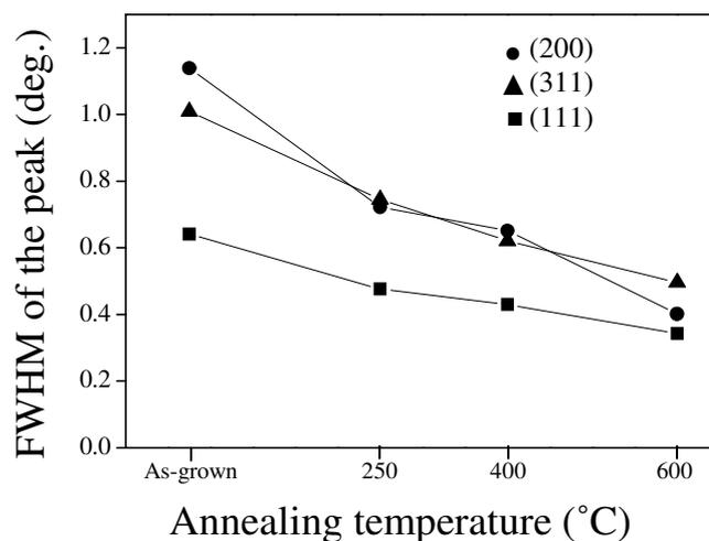
Fig. 4. Variation of the full width at half-maximum (FWHM) of the Au diffraction peaks by varying the annealing temperature.
