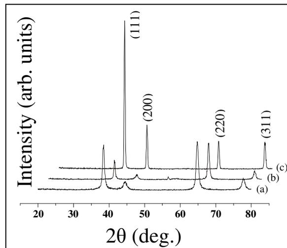
Fig. 3. X-ray diffraction patterns of Au thin films on Si substrate (a) without annealing and with annealing (b) at 250°C and (c) at 600°C.
