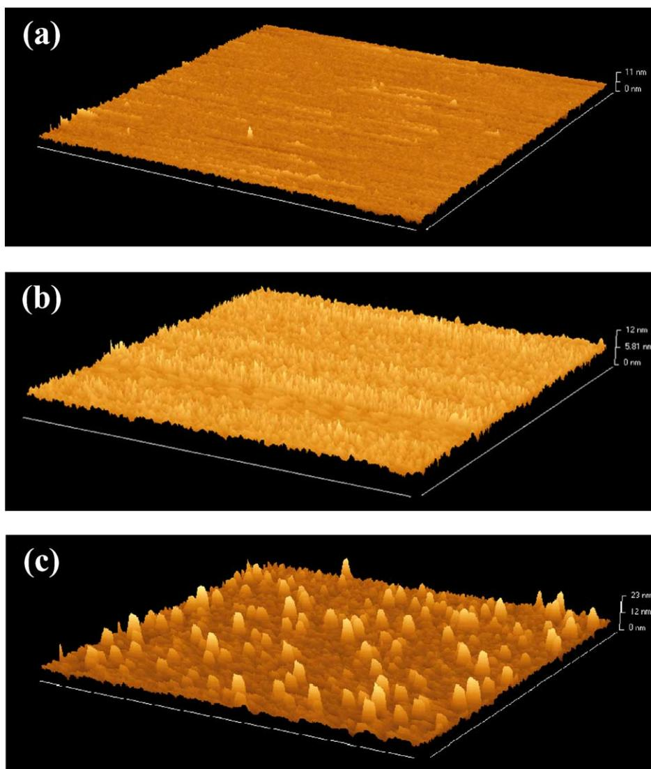
Fig. 1. AFM topographies of (a–c) GaN film surfaces and (d–f) ZnO buffer layer surfaces. The thicknesses of ZnO buffer layers are: (a, d) 20 nm; (b, e) 60 nm; and (c, f) 300 nm.
