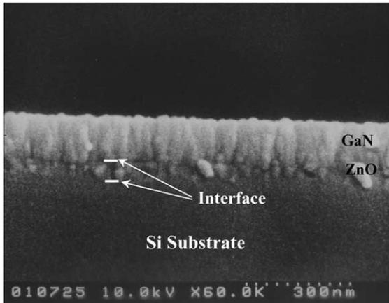
Fig. 4. Cross-sectional SEM image of GaN film when the ZnO buffer layer thickness is 60 nm.
