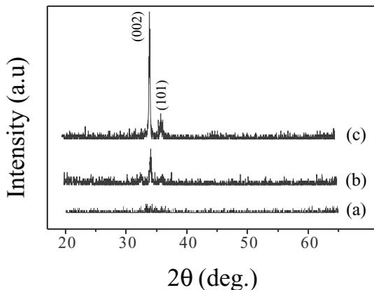
Fig. 5. XRD patterns of the GaN thin film deposited on ZnO/Si, with the ZnO buffer layer thicknesses of: (a) 20 nm; (b) 60 nm; and (c) 300 nm.
