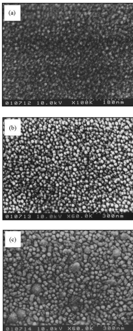
Fig. 3. Plain-view SEM images of GaN film with the ZnO buffer layer thickness of: (a) 20 nm; (b) 60 nm; and (c) 300 nm.
