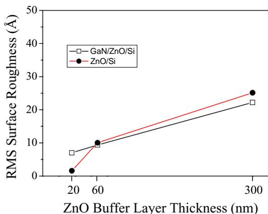
Fig. 2. AFM RMS surface roughness of GaN layer and ZnO buffer layer surfaces by varying the ZnO buffer layer thickness.
