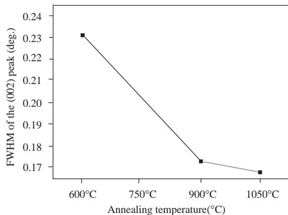
Fig. 2. Variation of the FWHM of the (002) diffraction peak by varying the annealing temperature in an ambient of oxygen.
