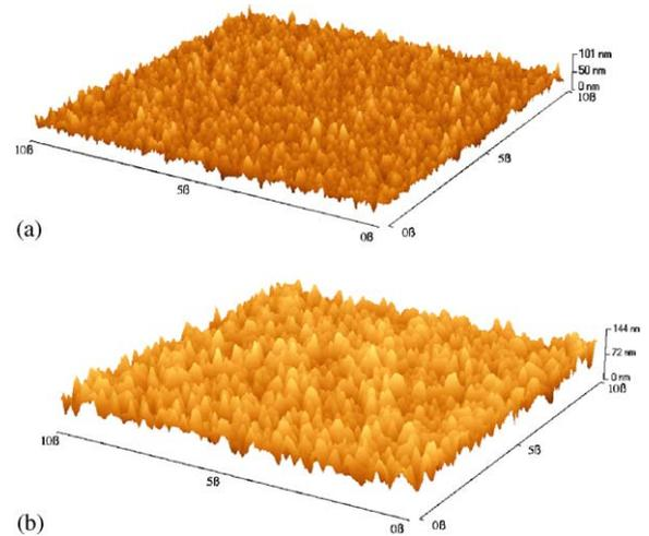
Fig. 6. AFM images of ZnO thin films annealed (a) at 600°C and (b) at 1050°C.
