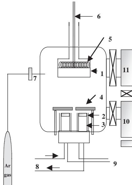
1. Substrate 2. Target 3. Magnetron 4. Shutter 5. Heater
