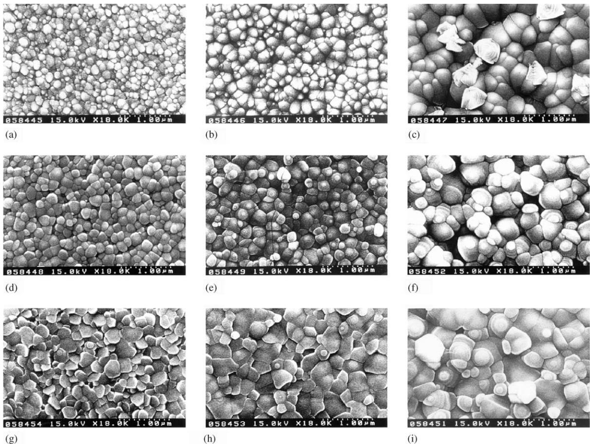
Fig. 7. Plain-view SEM images of ZnO film grown at room temperature with the annealing temperature of (a,b,c) 600°C, (d,e,f) 900°C and (g,h,i) 1050°C. The original thicknesses of ZnO films are (a,d,g) 400 nm, (b,c,h) 800 nm and (c,f,i) 1300 nm.
