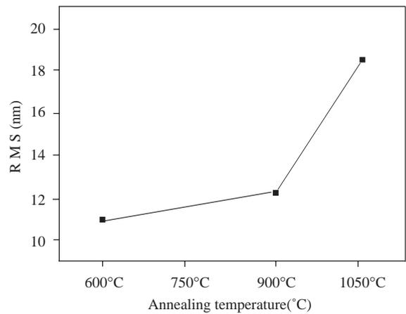
Fig. 5. Variation of RMS roughness measured by AFM, by varying the annealing temperature.
