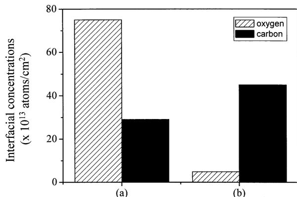
Figure 2 Column bar graph representing the oxygen and carbon concentration of the epilayer/substrate interfaces, based on SIMS data, (a) with spin drying and (b) with blow drying. The wafers were rinsed in DI water and *in-situ* cleaned at 600 °C.
