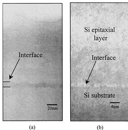
Figure 1 Cross-sectional TEM images of the epilayer/substrate interfaces (a) with spin drying and (b) with blow drying. The wafers were rinsed in DI water and *in-situ* cleaned at 600 °C.
