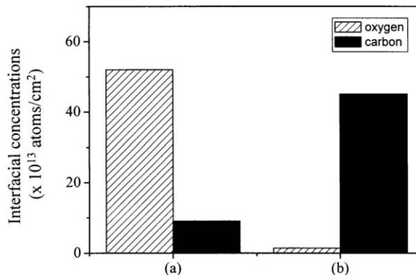
Figure 4 Column bar graph representing the oxygen and carbon concentration of the epilayer/substrate interfaces, based on SIMS data, (a) without and (b) with blow drying. The Si films are deposited at 660 °C without rinsing and an *in-situ* cleaning.
