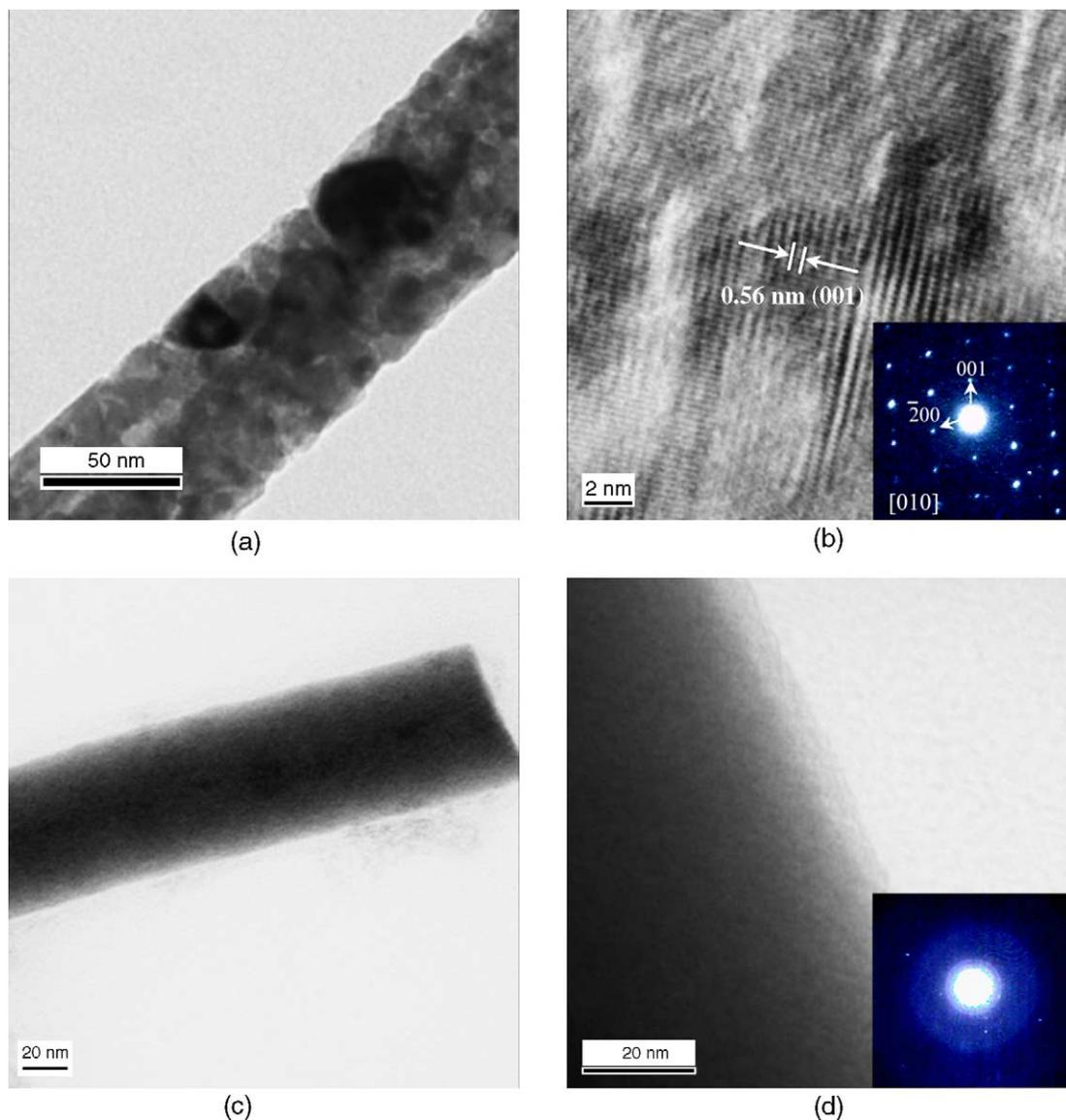
Fig. 5. TEM characterization of the gallium oxide nanowires with a (a, b) rough and (c, d) smooth surface. (a, c) Low magnification TEM image; (b, d) high resolution TEM image (inset: corresponding electron diffraction pattern).
