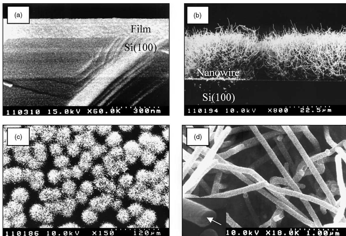
Fig. 2. SEM images of gallium oxide deposits grown on Si(1 0 0) substrate when the Ar/O<sub>2</sub> gas flow ratios are (a) 3 and (b)–(d) 5. (b) Cross-sectional image; (c) plain-view image; (d) high-magnification images (inset: magnified image of a deposit, exhibiting the circular cross-section).
