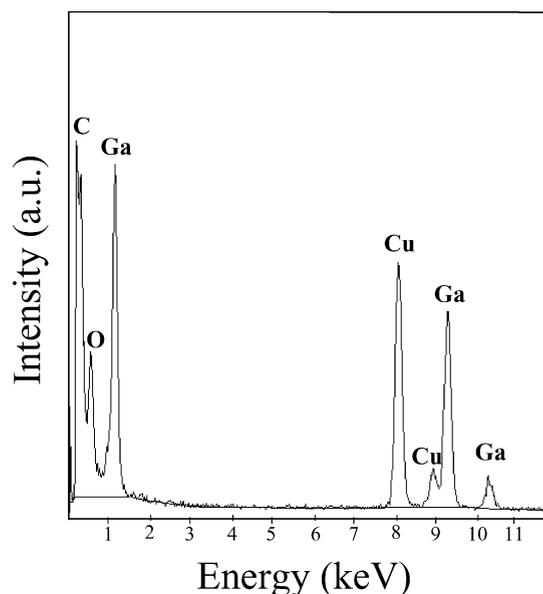
Fig. 4. A typical EDS spectrum of the 1D gallium oxide deposits grown on Si(1 0 0) substrate. The Cu and C peaks come from the supporting carbon-coated copper grids in TEM sample preparation.
