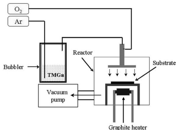
Fig. 1. Schematic illustration of the MOCVD reactor.
