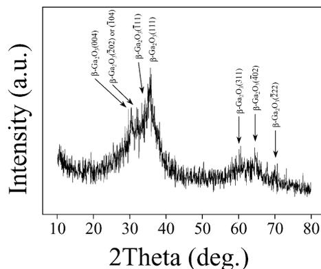
Fig. 3. X-ray diffraction patterns recorded from 1D gallium oxide deposits.
