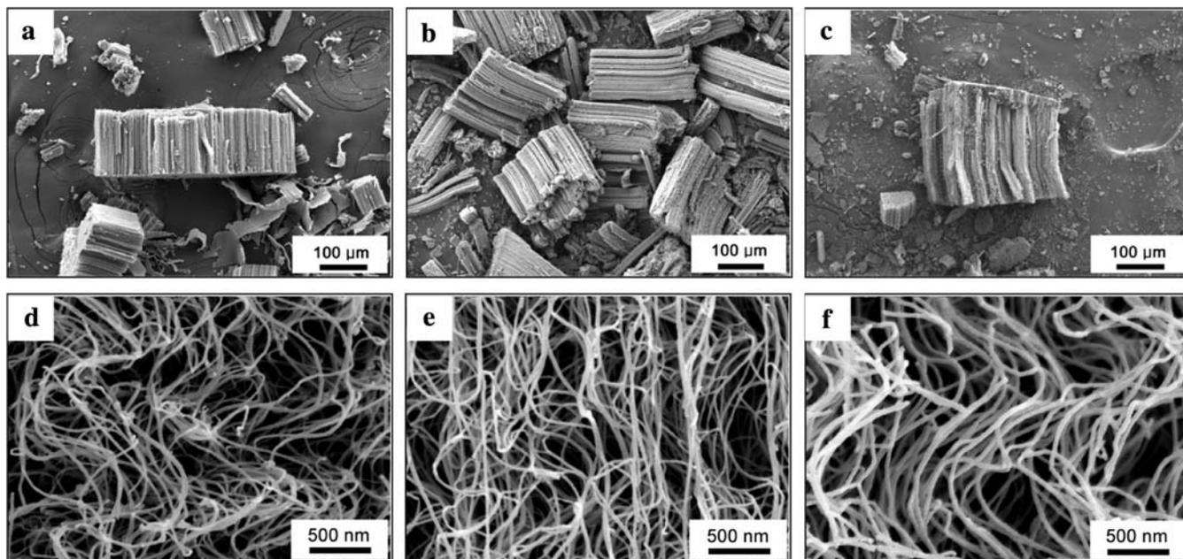
**FIGURE 1** SEM images of CNTs synthesized at 750–950 °C for 30 min. SEM image of CNTs grown at 750 °C (a, d); 850 °C (b, e); and 950 °C (c, f)
