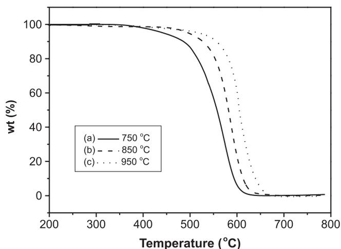
**FIGURE 3** TGA data of weight loss in percentage vs oxidation temperature for the CNTs grown at: **a** 750 °C; **b** 850 °C; and **c** 950 °C
