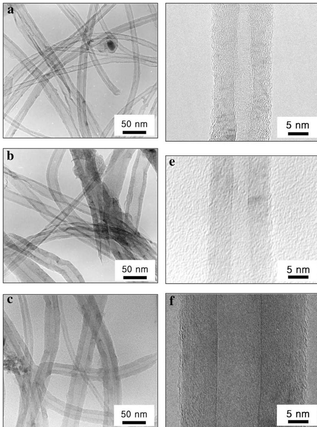
**FIGURE 2** TEM images of the CNTs **a**, **b** and **c** at low magnification and **d**, **e** and **f** at high magnification, grown at different temperatures: 750 °C (**d**); 850 °C (**e**); and 950 °C (**f**)
