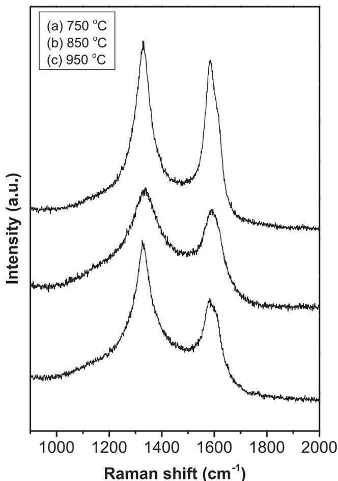
**FIGURE 4** Raman spectra of CNTs grown at: **a** 750 °C; **b** 850 °C; and **c** 950 °C. The peak intensity ratio of D- and G-bands decreases with increasing the growth temperature
