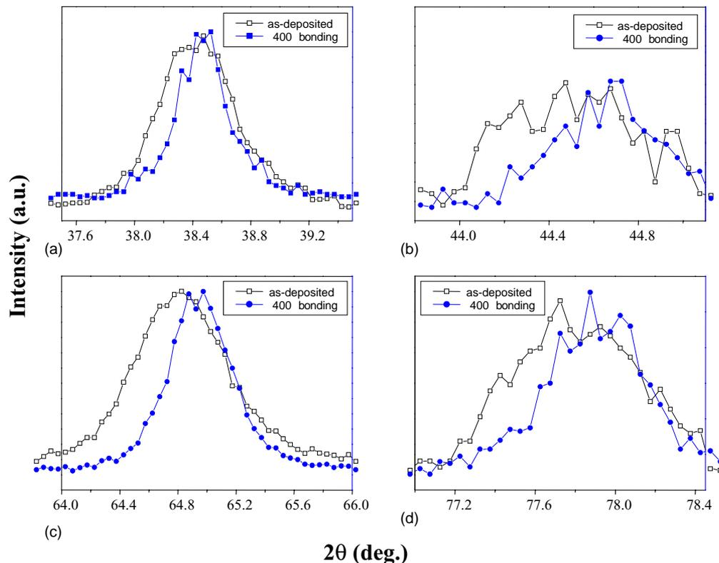
Fig. 5. Portions of X-ray diffraction spectra, revealing the (a) (1 1 1), (b) (2 0 0), (c) (2 2 0), and (d) (3 1 1) diffraction peaks of as-deposited and 400 °C-bonded layers.
