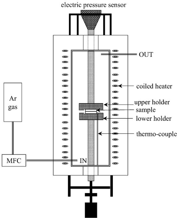
Fig. 1. Schematic diagram of a vertical furnace used for the wafer bonding.
