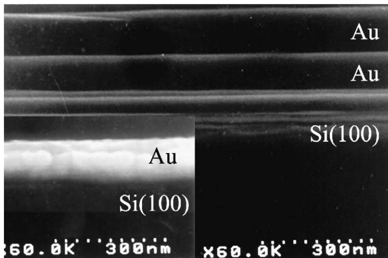
Fig. 2. Cross-sectional SEM images of Au–Au-bonded layer at 400 °C (Inset: cross-sectional SEM images of as-deposited Au layer).
