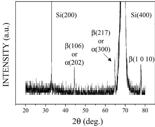
Fig. 1. XRD patterns recorded from Ga<sub>2</sub>O<sub>3</sub> deposits at 550 °C. Indexing of weak diffraction peaks corresponds to a monoclinic structure of β-Ga<sub>2</sub>O<sub>3</sub> and/or a hexagonal corundum structure of α-Ga<sub>2</sub>O<sub>3</sub>.
