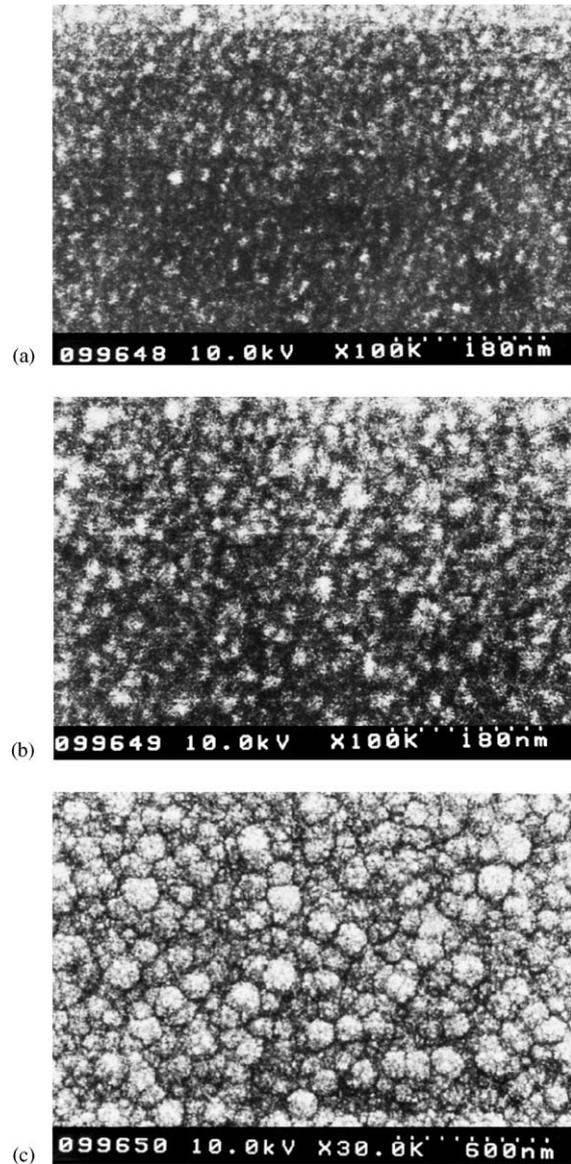
Fig. 4. Plain-view SEM images of Ga<sub>2</sub>O<sub>3</sub> films at a growth temperature of (a) 500 °C, (b) 550 °C, and (c) 600 °C.
