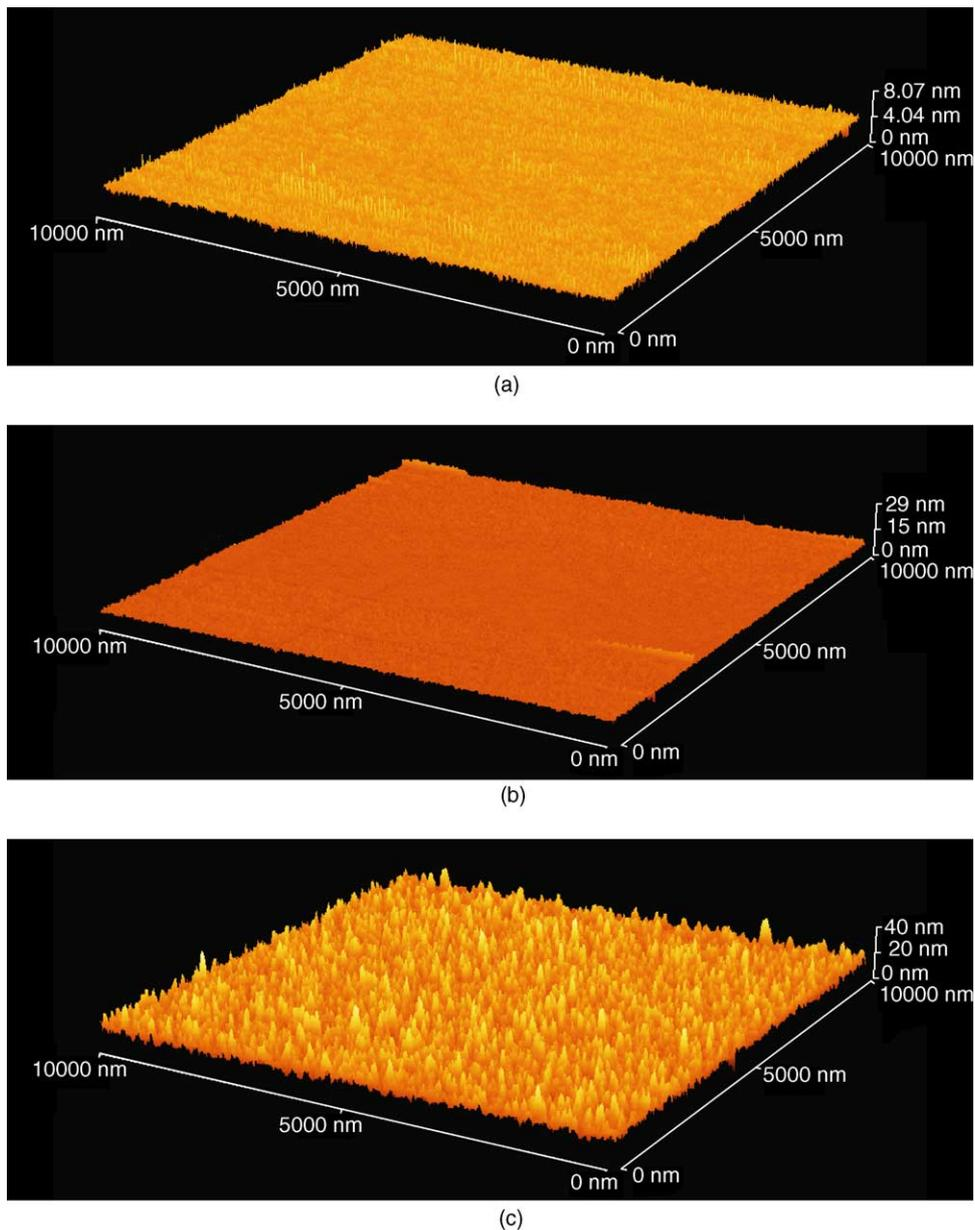
Fig. 5. AFM images of Ga<sub>2</sub>O<sub>3</sub> films at a growth temperature of (a) 500 °C, (b) 550 °C, and (c) 600 °C.
