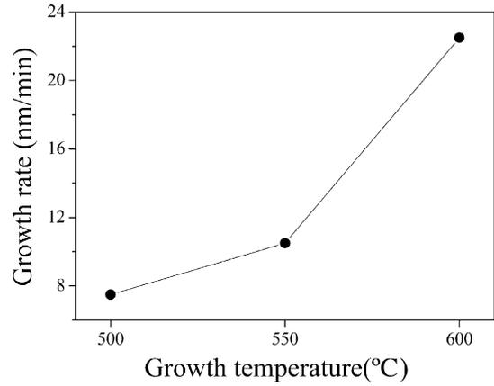
Fig. 3. Dependence of film growth rate on the substrate temperature, indicating that the growth rate increases with increasing the growth rate.
