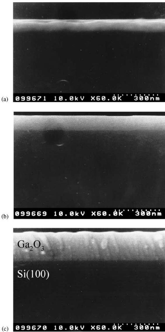
Fig. 2. Cross-sectional SEM images of Ga<sub>2</sub>O<sub>3</sub> films at a growth temperature of (a) 500 °C, (b) 550 °C, and (c) 600 °C.
