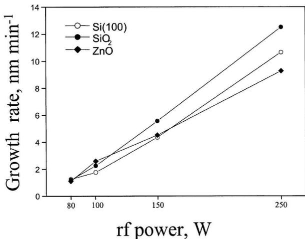
1 Dependence of ZnO film growth rate on rf power and substrate material
