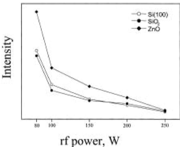
2 Relative intensity of ZnO films deposited on given substrates as function of rf power
