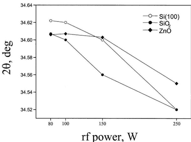
3 XRD peak angles of ZnO films deposited on given substrates as function of rf power
