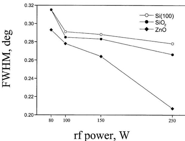
5 Full width at half maximum of ZnO films deposited on given substrates as function of rf power
