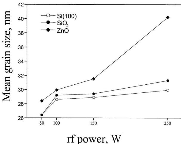
6 Mean grain size of ZnO films deposited on given substrates as function of rf power: grain size calculated using Scherrer formula
