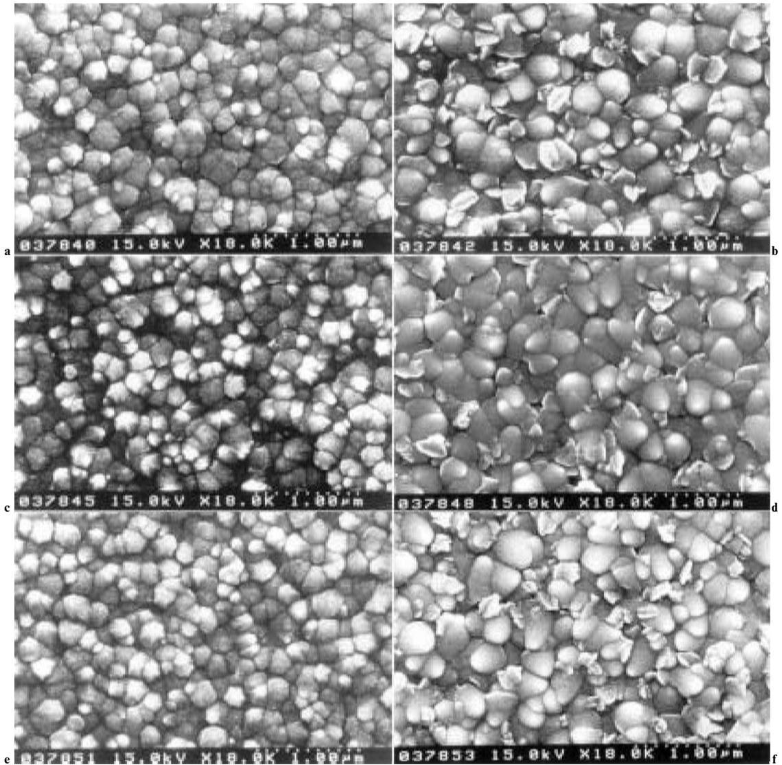
7 Plain view SEM images of ZnO thin films deposited on *a,b* Si(100), *c,d* SiO<sub>2</sub>, *e,f* amorphous ZnO substrates at room temperature, at rf powers of 100 W (*a,c,e*) and 250 W (*b,d,f*)
