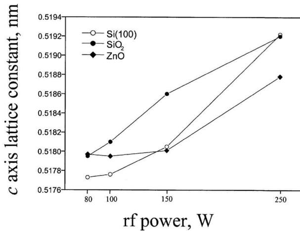
4 Variation of *c* axis lattice constant of ZnO films deposited on given substrates as function of rf power
