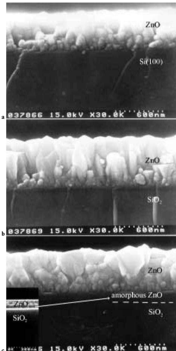
**8** Cross-sectional SEM images of ZnO thin films deposited on *a* Si(100), *b* SiO<sub>2</sub>, *c* amorphous ZnO substrates at room temperature, at rf power of 150 W: inset shows amorphous ZnO layer before ZnO deposition
