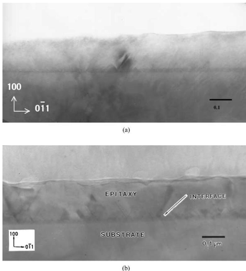
Figure 1 XTEM image of samples with different interfacial carbon concentrations, revealing that the crystallinity of silicon epitaxial layer is not improved by reducing the carbon interfacial concentration. The interfacial carbon concentrations are (a)  $1.1 \times 10^{14}$  and (b)  $1.5 \times 10^{13}$ , respectively.
