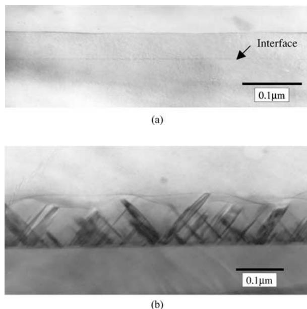
Figure 2 XTEM image of samples with different interfacial oxygen concentrations, revealing that the crystallinity of silicon epitaxial layer is degraded by increasing the oxygen interfacial concentration. The interfacial oxygen concentrations are (a)  $7.8 \times 10^{14}$  and (b)  $1.8 \times 10^{15} \text{ cm}^{-2}$ , respectively.
