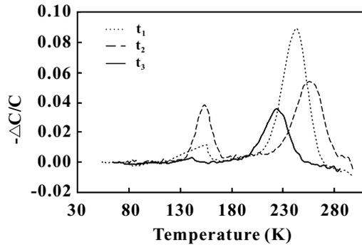
Fig. 7. The DLTS spectra of the silicon substrate irradiated by 12 MeV electron with a dose of 800 kgy.
