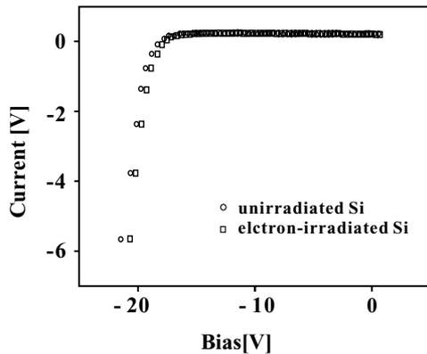
Fig. 4. Current–voltage ( $I$ – $V$ ) characteristics of the electron-irradiated and unirradiated p–n junction diodes under the reverse bias.
