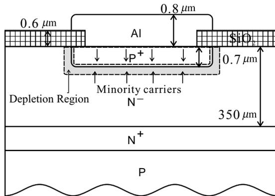
Fig. 1. Schematic diagram of a p–n junction diode structure.
