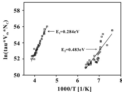
Fig. 8. The Arrhenius plots for the DLTS analysis results shown in Fig. 7.
