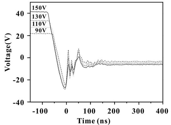
Fig. 2. Voltages measured at various forward injections for the p–n junction diode.
