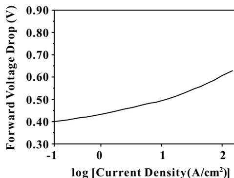
Fig. 5. Difference in forward voltage drop of the p–n junction diode as a function of the current density due to electron irradiation and subsequent annealing.
