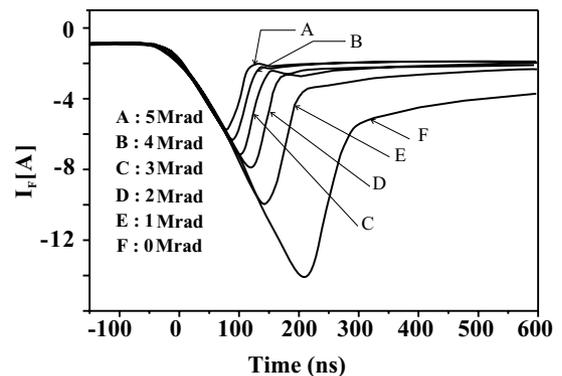
Fig. 3. The recovery current waveforms of the p–n junction diode irradiated by 12 MeV electrons with different doses.
