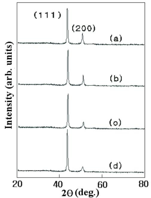
Fig. 8. X-ray diffraction patterns of the copper films after vacuum furnace annealing for 5 minutes at different temperature (a) 200 °C, (b) 300 °C, (c) 400 °C, and (d) 500 °C.
