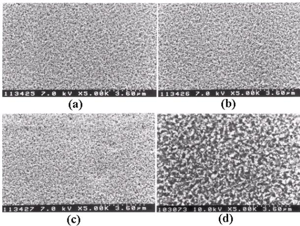
Fig. 7. Scanning electron micrographs of the copper films after rapid thermal nitriding for 15 sec at different temperature (a) 200 °C, (b) 300 °C, (c) 400 °C, and (d) 500 °C.
