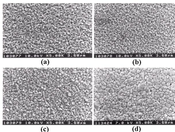
Fig. 5. Scanning electron micrographs of the copper films after vacuum furnace annealing for 5 minutes at different temperature (a) 200 °C, (b) 300 °C, (c) 400 °C, and (d) 500 °C.
