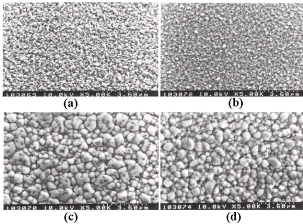
Fig. 6. Scanning electron micrographs of the copper films after rapid thermal annealing (RTA) for 15 sec at different temperature (a) 200 °C, (b) 300 °C, (c) 400 °C, and (d) 500 °C.
