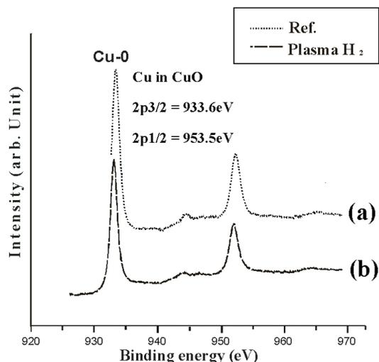
Fig. 4. The XPS  $Cu2p$  peaks of the Cu seed: (a) reference (b) plasma hydrogen pretreatment (100 W, 10 min.) of the Cu seed layer.
