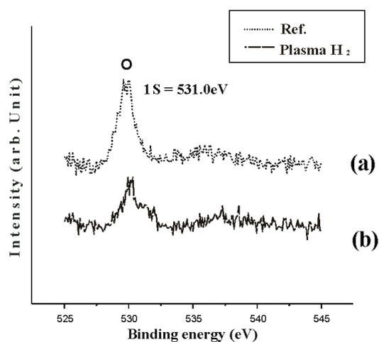
Fig. 3. The XPS  $O1s$  peak (531.0 eV) of the Cu seed: (a) reference (b) plasma hydrogen pretreatment (100 W, 10 min.) of the Cu seed layer.
