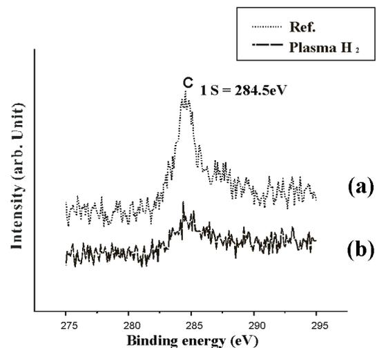
Fig. 2. The XPS C1s peak (284.5 eV) of the Cu seed: (a) reference (b) H<sub>2</sub> plasma pretreatment (100 W, 10 min.) of the Cu seed layer.
