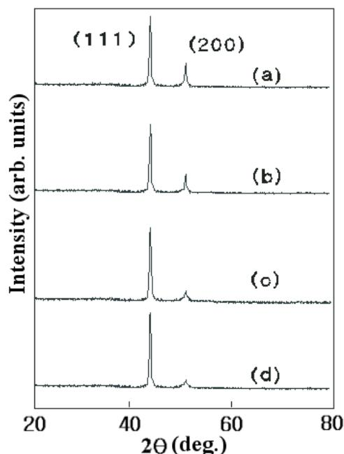
Fig. 10. X-ray diffraction patterns of the copper films after rapid thermal nitriding for 15 sec at different temperature (a) 200 °C, (b) 300 °C, (c) 400 °C, and (d) 500 °C.
