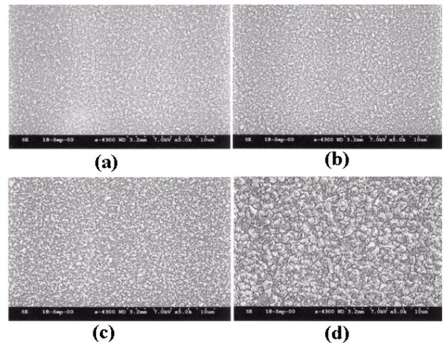
Fig. 1. SEM micrographs ( $\times 5000$ ) of the electroplated copper films after the plasma pretreatment of the Cu seed layer at various rf-powers (exposure time: 10 min.): (a) 20 W, (b) 60 W, (c) 100 W and (d) 140 W.
