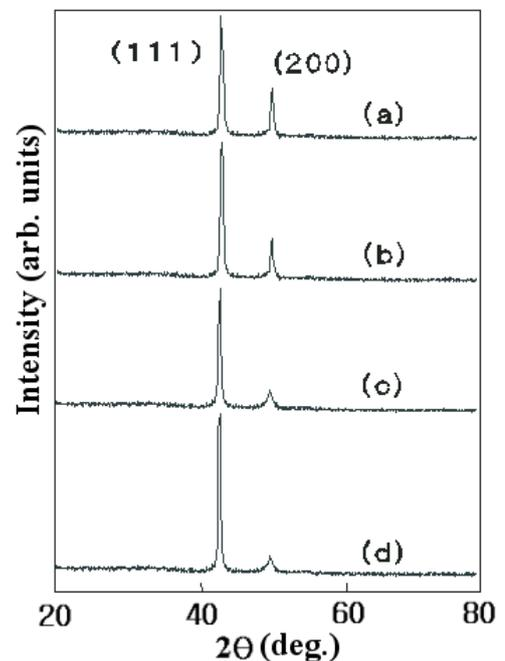
Fig. 9. X-ray diffraction patterns of the copper films after rapid thermal annealing (RTA) for 15 sec at different temperature (a) 200 °C, (b) 300 °C, (c) 400 °C, and (d) 500 °C.
