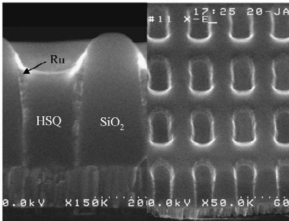
Fig. 3. SEM images of the concave-type structure after the etchback of Ru bottom electrode layer.
