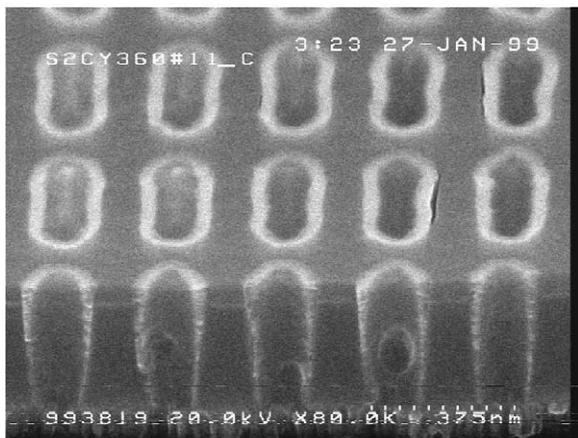
Fig. 6. SEM image of the concave-type structure after removing the HSQ with the HF solution. There is no spacing between the  $\text{SiO}_2$  and the Ru, due to the insertion of a  $\text{Ta}_2\text{O}_5$  layer.
