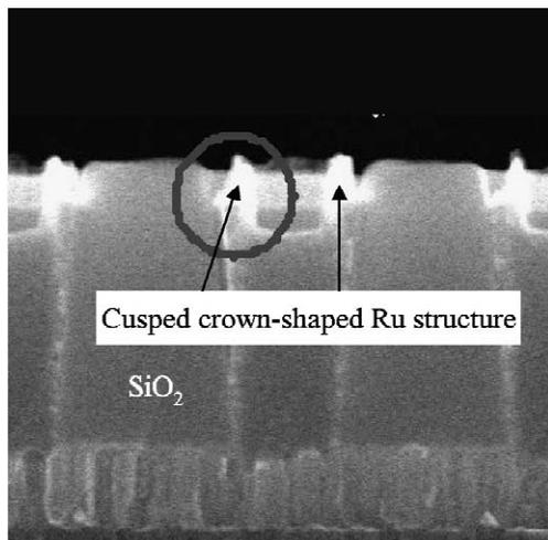
Fig. 4. SEM image of the concave-type structure after the etchback of the Ru bottom electrode layer, indicating that the cusped crown-shaped structure is generated due to insufficient removal of the HSQ layer.
