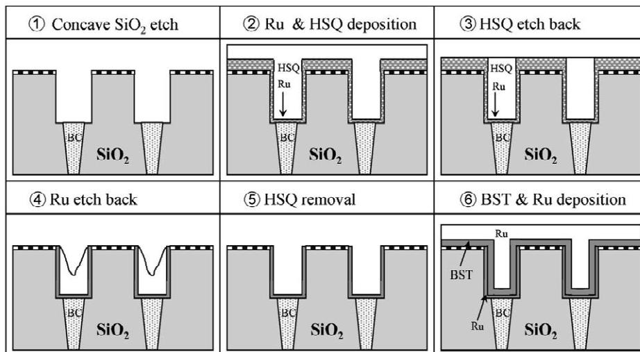
Fig. 1. The fabrication sequence of concave-type Ru/BST/Ru capacitor ('BC' represents the buried contact).
