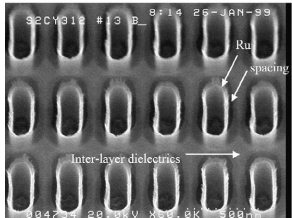
Fig. 5. SEM image of the concave-type structure with the cusped crown-shaped Ru after removing the HSQ with the HF solution.
