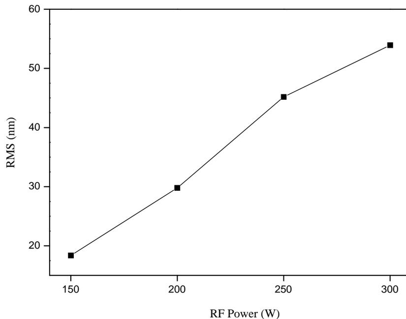
Fig. 2. AFM RMS roughness values of ZnO thin film on Si(001) substrate deposited at room temperature with the RF power ranging from 150 to 300 W.
