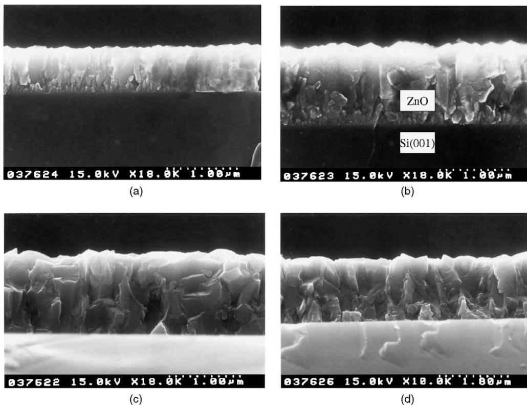
Fig. 5. Cross-sectional SEM images of the ZnO thin film deposited with the RF power of (W): (a) 150, (b) 200, (c) 250, and (d) 300.
