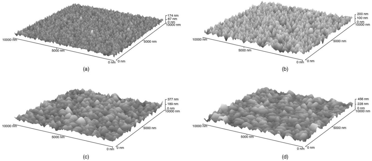
Fig. 3. Images of the ZnO thin film deposited with the RF power of (W): (a) 150, (b) 200, (c) 250, and (d) 300.
