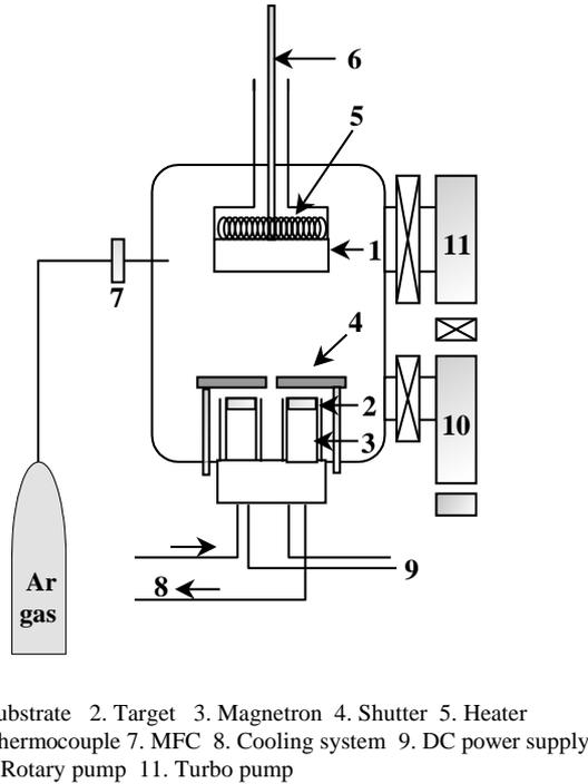
Fig. 1. Schematic diagram of RF magnetron sputtering system.
