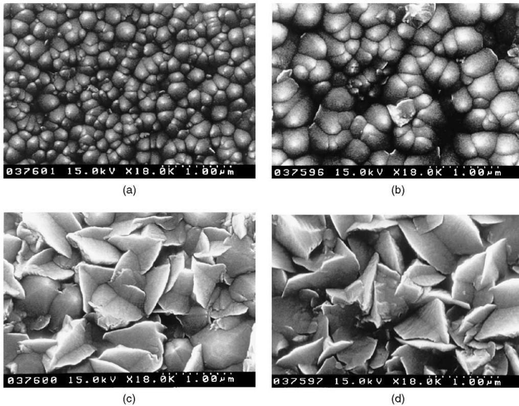
Fig. 4. Plain-view SEM images of the ZnO thin deposited with the RF power of (W): (a) 150, (b) 200, (c) 250, and (d) 300.
