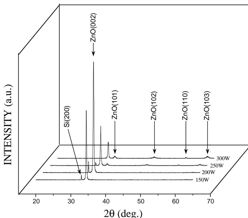
Fig. 6. XRD patterns of the ZnO thin film deposited with varying RF power ranging from 150 to 300 W.
