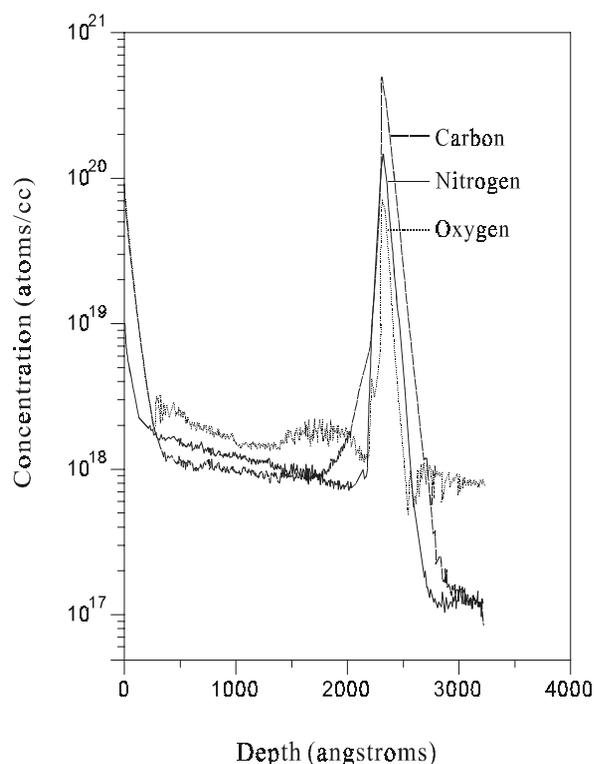
Figure 2 SIMS depth profile of epitaxial film and the interface, *in-situ* cleaned with a microwave power of 300 W, DC bias of 10 V, pressure of 1 mTorr, and the cleaning temperature of 600 °C.
