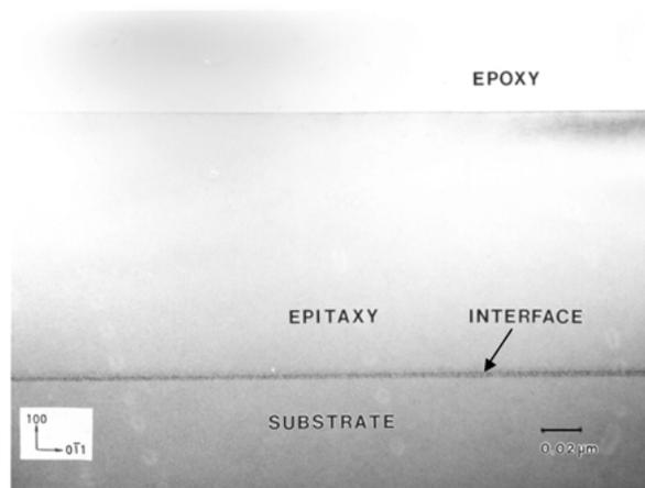
Figure 1 XTEM image of silicon epilayer and the interface, *in-situ* cleaned with a microwave power of 300 W, DC bias of 10 V, pressure of 1 mTorr, and the cleaning temperature of 600 °C. The high-quality epitaxial layer is produced by applying the *in-situ* plasma cleaning.
