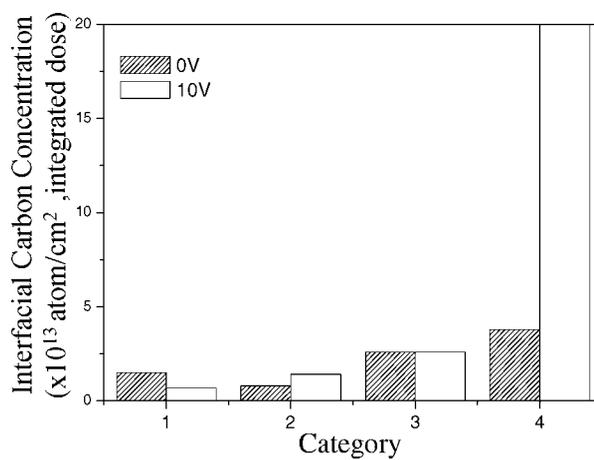
Figure 4 Column bar graph showing the effect of substrate DC bias on the interfacial carbon concentration.
