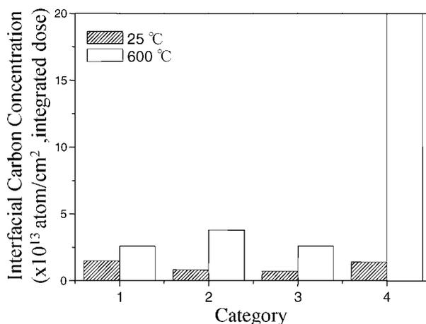
Figure 3 Column bar graph showing the effect of cleaning temperature on the interfacial carbon concentration.
