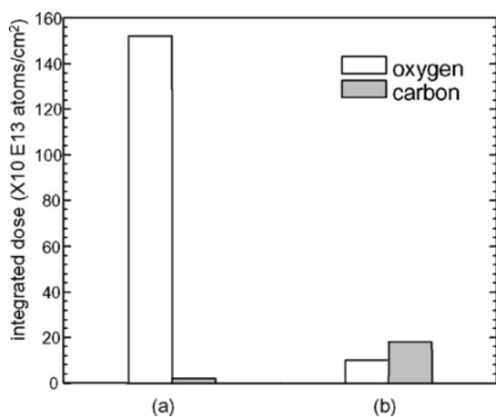
Figure 2 Column bar graph showing the effect of *in-situ* cleaning and growing temperature on the interfacial oxygen and carbon concentration. The *in-situ* cleaning and deposition temperature is set to (a) 550 °C and (b) 660 °C.
