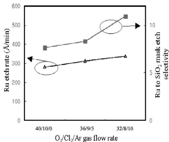
Fig. 2. Change of Ru etch rate, Ru to  $SiO_2$  etch selectivity depending on the  $O_2/Cl_2/Ar$  gas flow ratio.
