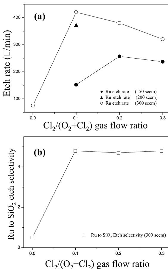
Fig. 1. (a) Change of Ru etch rate by varying  $\text{Cl}_2/(\text{O}_2 + \text{Cl}_2)$  gas flow ratio, Pressure ranges from 50 to 300 sccm. (b) Change of Ru to  $\text{SiO}_2$  etch selectivity by varying  $\text{Cl}_2/(\text{O}_2 + \text{Cl}_2)$  gas flow ratio at a pressure of 300 sccm.
