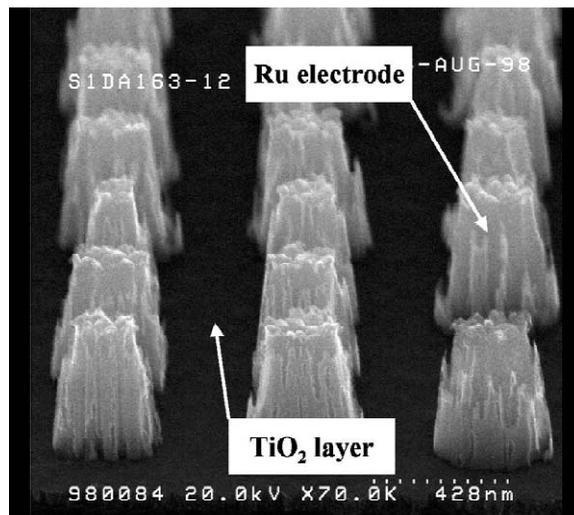
Fig. 4. SEM images of Ru etching profile with the bottom layer of  $\text{TiO}_2$ .
