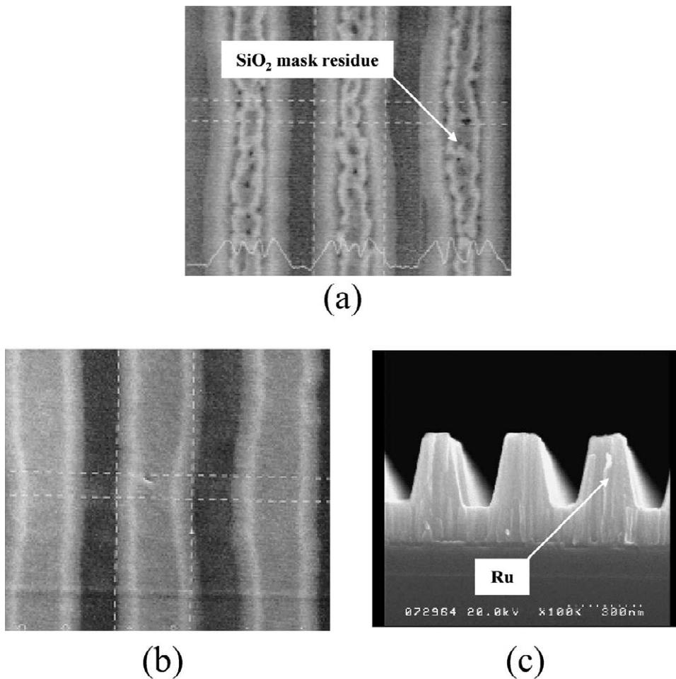
Fig. 5. SEM images of Ru gate patterns showing the removal of SiO<sub>2</sub> mask. (a) Top view of the patterns etched with a low (250 W) RF power. (b) Top view of the patterns etched with a high (600 W) RF power. (c) Cross-sectional view of the patterns etched with a high (600 W) RF power.
