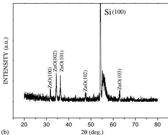
Fig. 3. (a) SEM images and (b) X-ray rocking curves of ZnO nanorods grown directly on silicon substrate at 500°C.
