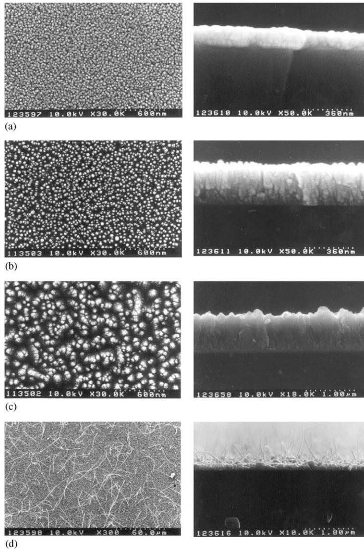
Fig. 2. SEM images of top view (left) and cross-sectional view (right) of ZnO films deposited at (a) 250°C, (b) 300°C, (c) 400°C, and (d) 500°C.
