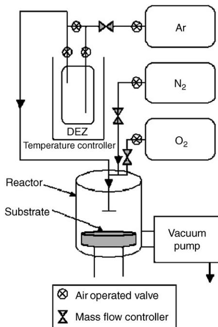
Fig. 1. Schematic diagram of the MOCVD system.
