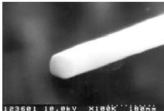
Fig. 4. SEM image of a ZnO nanorod, indicating a diameter of 110 nm.
