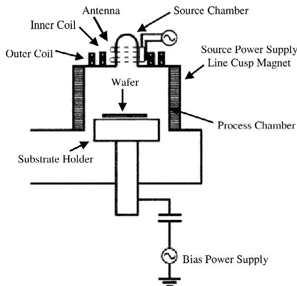
Fig. 1. Schematic diagram of an  $m = 0$  helicon plasma reactor.
