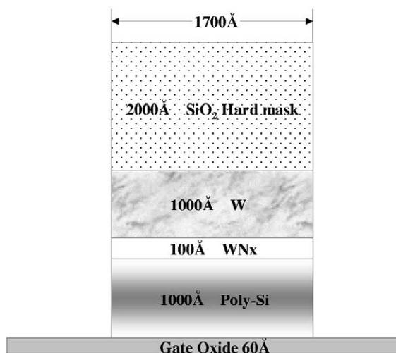
Fig. 2. Cross-sectional view of gate electrode pattern with a SiO<sub>2</sub> hard mask 2000 Å/W 1000 Å/WN<sub>x</sub> 100 Å/poly-Si 1000 Å/gate oxide 60 Å.
