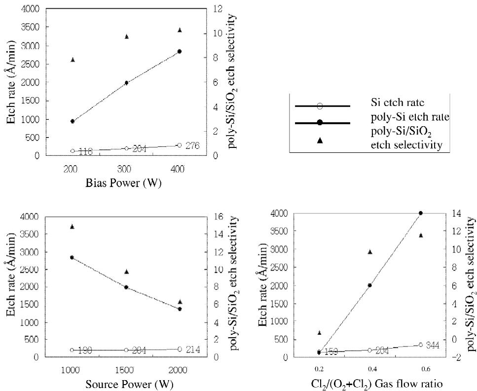
Fig. 5. Variation of the etch selectivity of poly-Si over SiO<sub>2</sub> with varying process parameters. The etch selectivity increase with increasing bias power, decreasing source power, and decreasing O<sub>2</sub> ratio in the Cl<sub>2</sub>/O<sub>2</sub> system.
