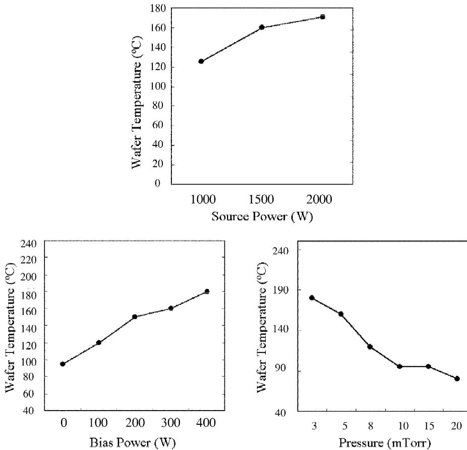
Fig. 6. Variation of the wafer temperature with varying process parameters.
