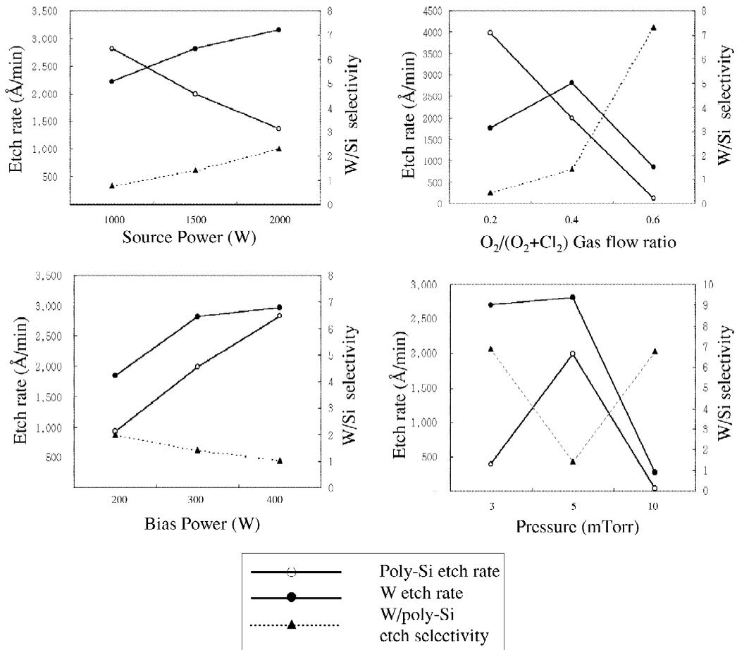
Fig. 3. Variation of W etch rates, poly-Si etch rate, and the etch selectivity of W over poly-Si with varying process parameters. The etch selectivity increases with increasing source power, decreasing bias power, and increasing O<sub>2</sub>/Cl<sub>2</sub> ratio.
