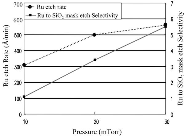
Fig. 4. Ru etch rates and Ru to SiO<sub>2</sub> mask etch selectivities as a function of pressure.
