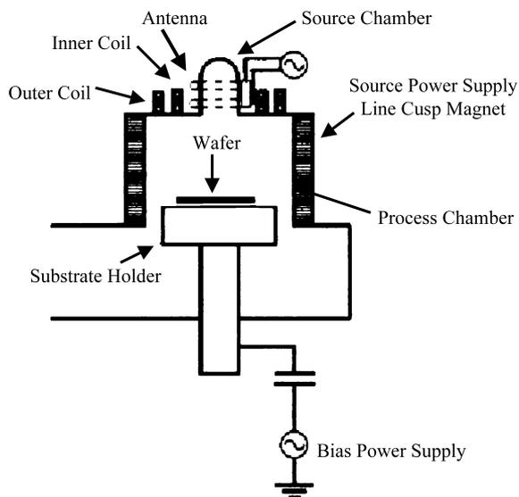
Fig. 1. Schematics diagram of a helicon chamber.
