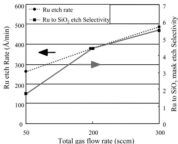
Fig. 3. Ru etch rates and Ru to  $SiO_2$  mask etch selectivities as a function of total gas flow rate.
