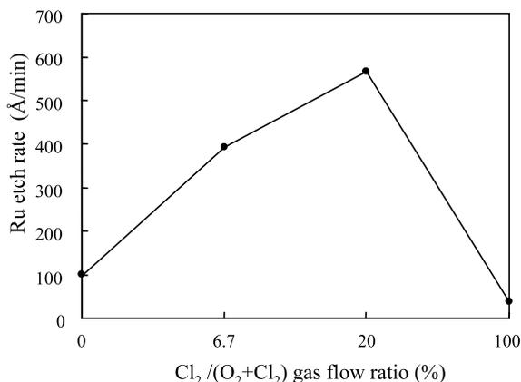
Fig. 2. Ru etch rates as a function of  $Cl_2/(O_2 + Cl_2)$  gas flow ratio.
