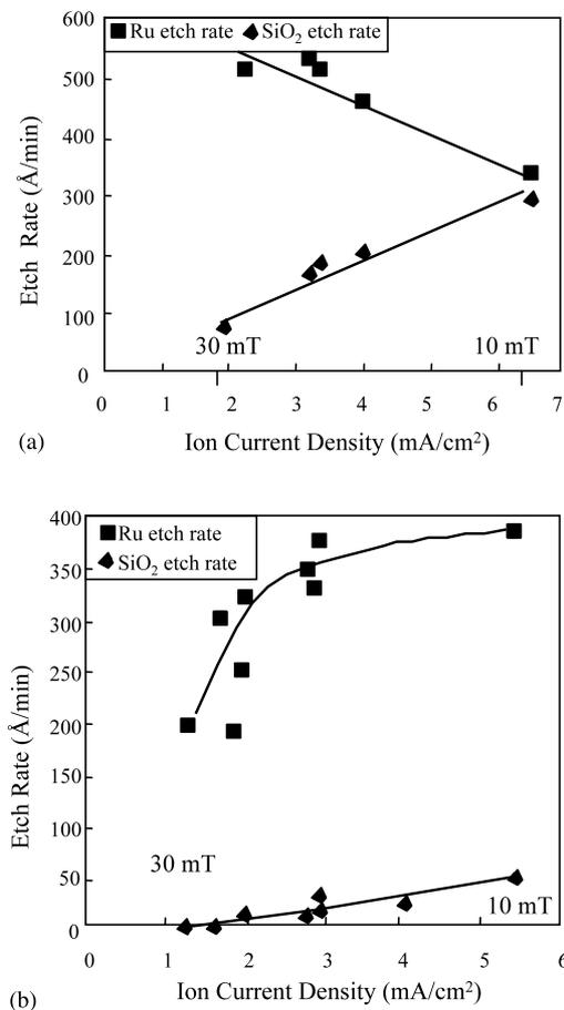
Fig. 7. Ru etch rate as a function of ion current density using (a) patterned wafers and (b) blanket wafers.
