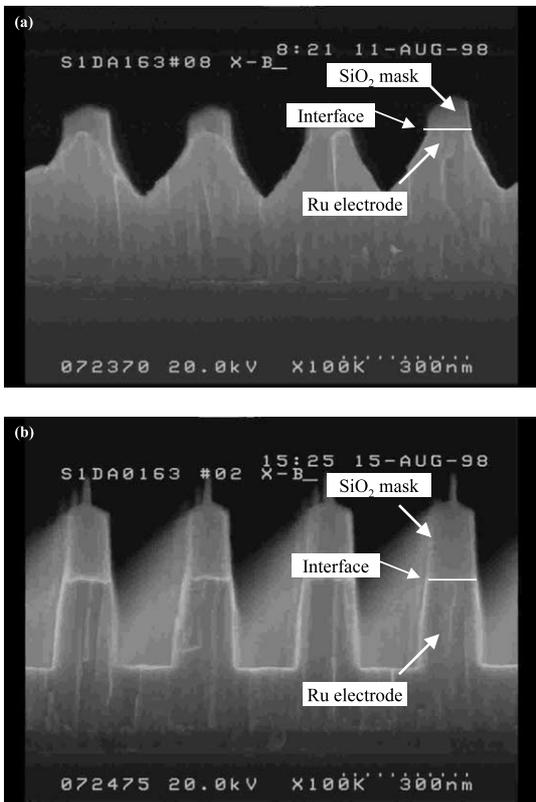
Fig. 5. Ru etching profile at (a) 10 and (b) 30 mTorr. The etching condition with the 20% of Cl<sub>2</sub>/(O<sub>2</sub>+Cl<sub>2</sub>) gas flow ratio, 300 sccm of total gas flow rate, 2000 W of source power, and 250 W of bias power, is applied.
