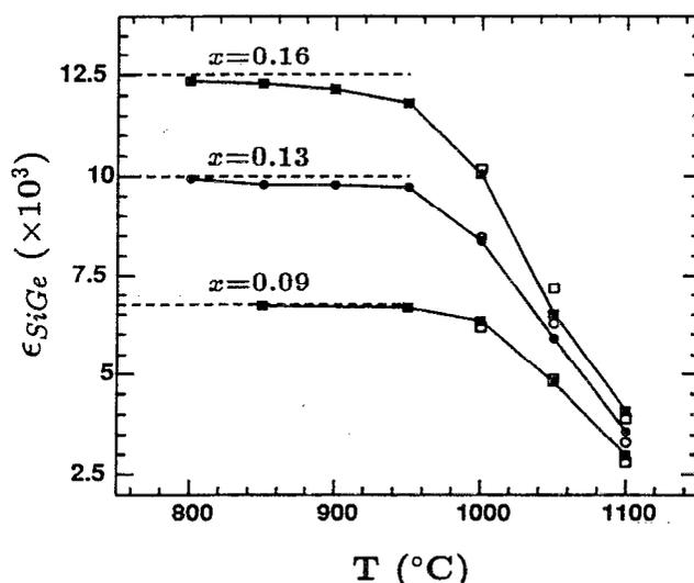
FIG. 1. Measured strain vs annealing temperatures for Ge=0.09, 0.13, and 0.16. The close symbols refer to the measured data, and the open symbols are from Eq. (4). The strains measured from as-grown samples are presented by the dashed lines.
