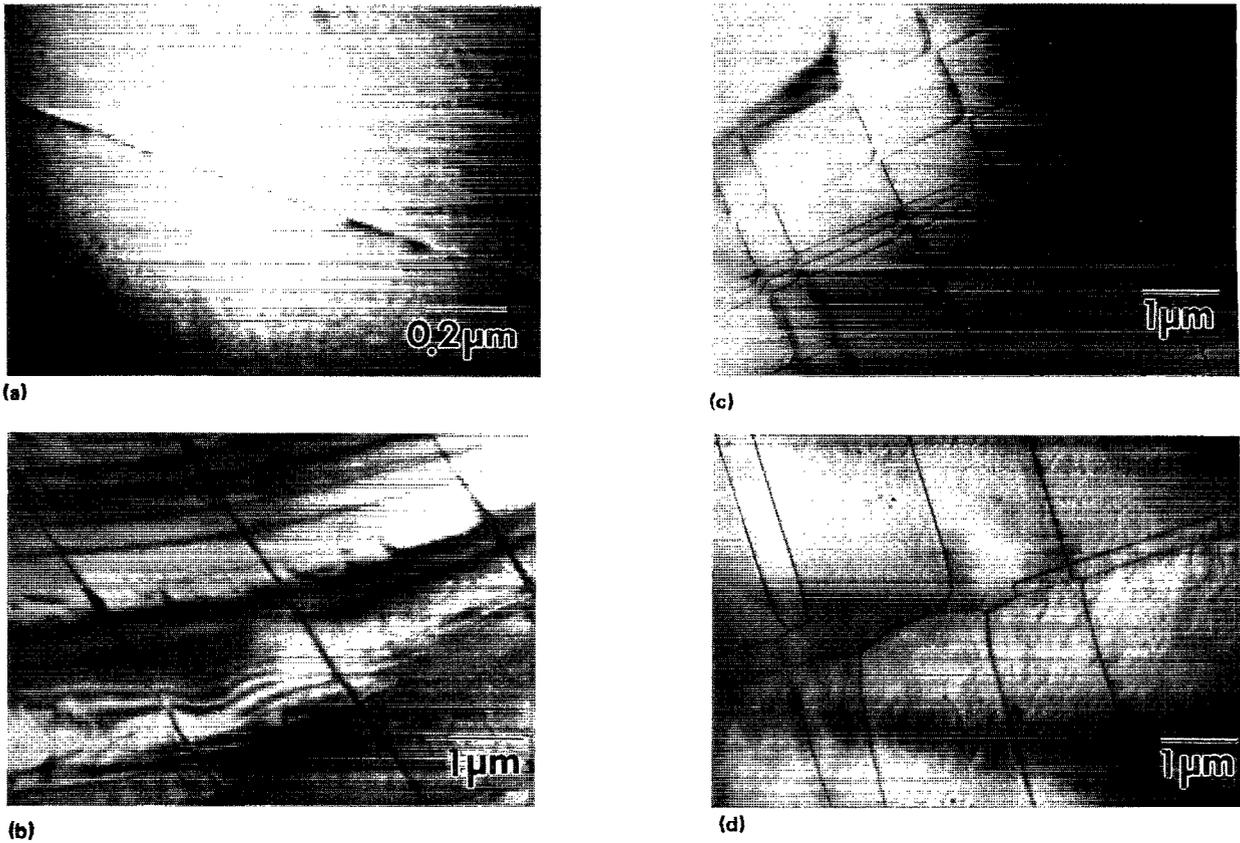
FIG. 2. Plan-view TEM micrographs of 1400 Å Si/550 Å Si<sub>0.87</sub>Ge<sub>0.13</sub>/Si annealed for 30 min at (a) 800 °C, (b) 900 °C, (c) 1000 °C, and (d) 1100 °C. Relaxation occurs only by single dislocations as  $\tau_{\text{eff}}^S = 2.2\tau_{\text{eff}}^P$ .
